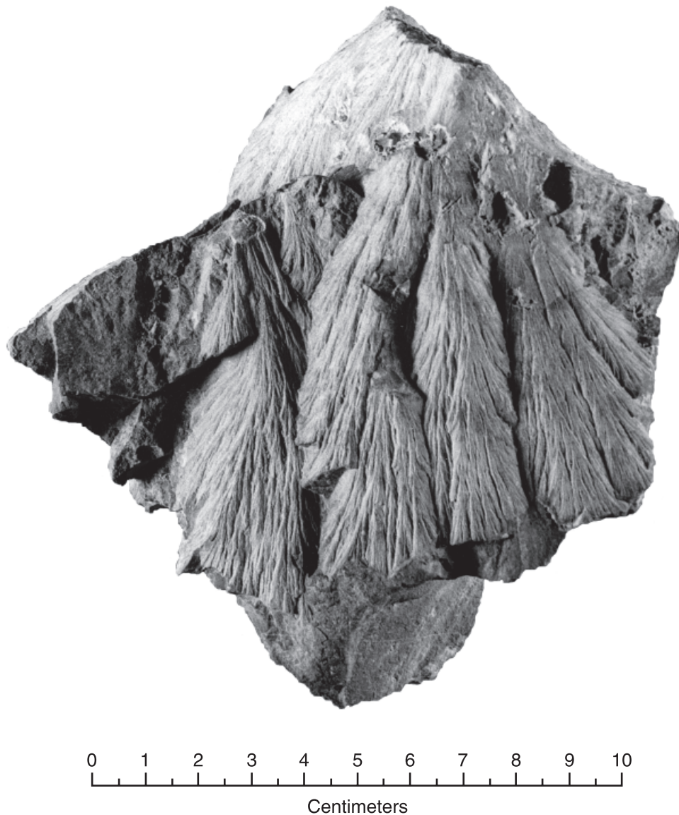
Fig. 4.6. Shatter cones; small, well-developed. Small, finely sculptured shatter cones, developed in fine-grained limestone from the Haughton structure (Canada). The cone surfaces show the typical divergence of striae away from the cone apex (“horsetailing”). Photograph courtesy of R. A. F. Grieve.
