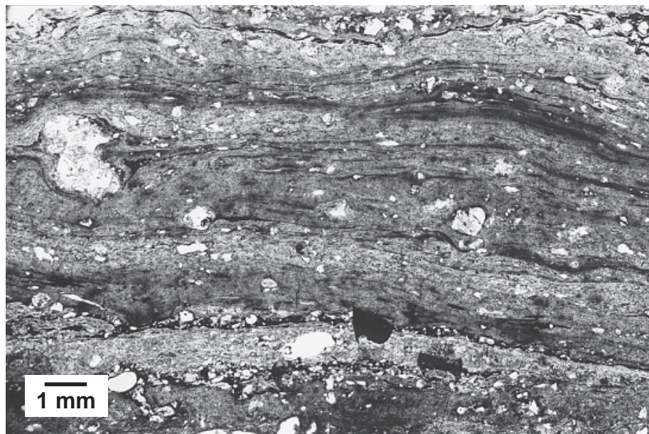
Fig. 5.11. Crater-fill breccia; suevite; glassy inclusion. Heterogeneous, fragment-rich glassy fragment ( Fladen ) in suevite breccia from Lake Mien (Sweden), showing complex, multiple layering with varying amounts of rock and mineral inclusions. The mineral inclusions are typically sharp to angular and do not show the phenocryst shapes that are typically observed in glassy volcanic rocks. The generally laminar flow-banding is emphasized by a sharp difference in clast content and by dark streaks that may represent decomposed and melted opaque minerals. Note that flow-banding in the clast-rich layers (e.g., top) is more highly contorted. Sample NBS-61-0487 (plane-polarized light).
