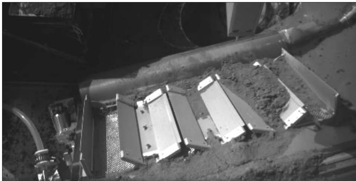
Martian soil on the doors of the Thermal and Evolved Gas Analyzer (TEGA), onboard the Phoenix Lander, October 7, 2008. (NASA/JPL-Caltech/University of Arizona/Max Planck Institute)
