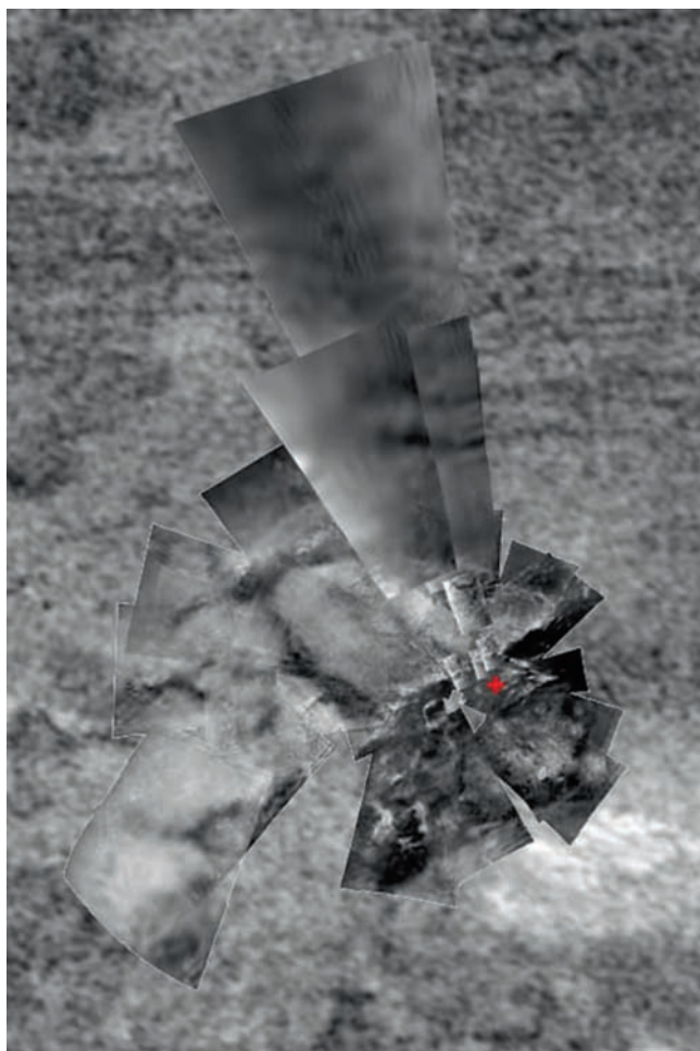
Fig. 5.41 Huygens landing site identification in T8 was facilitated by two dunes seen near the horizon in DISR SLI images north of the landing site indicated by (+). DISR mosaic overlaid on RADAR data. The image is about 100 km across
