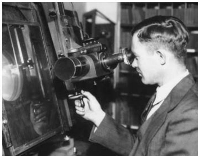
Clyde Tombaugh peers into a blink comparator at the Lowell Observatory, circa 1950. Such devices were used to check photographic plates for tiny, faint objects that moved between one exposure and another—objects such as Pluto.
