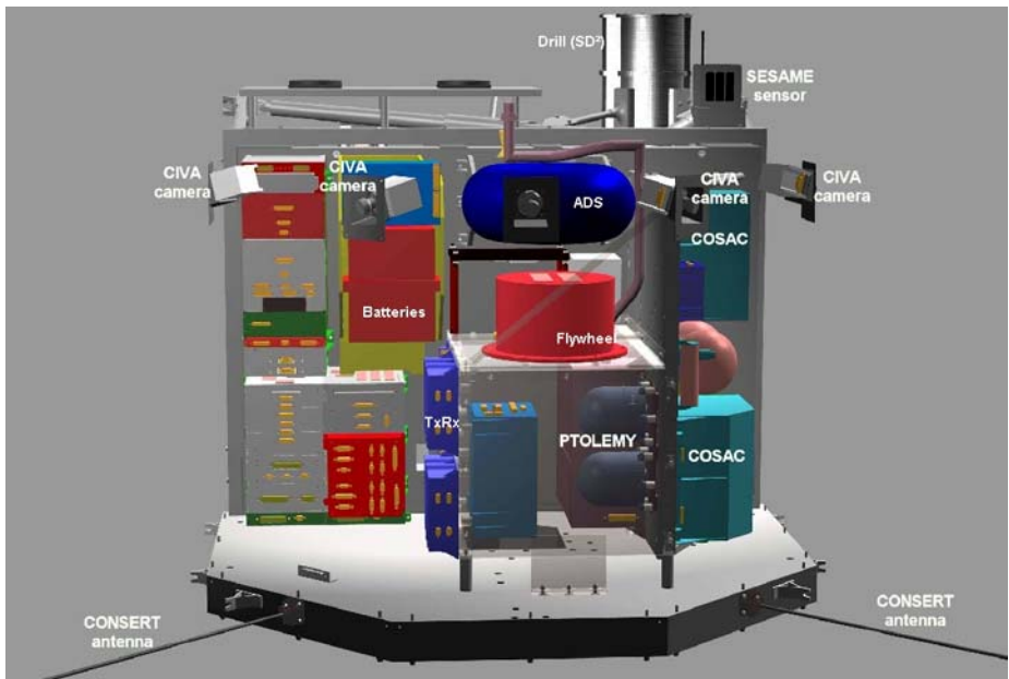
Fig. 5 Side view schematics of the inner structure of the lander compartment showing the location of COSAC and PTOLEMY systems, the CONSERT antennas, the SESAME dust sensor and various ÇIVA cameras
