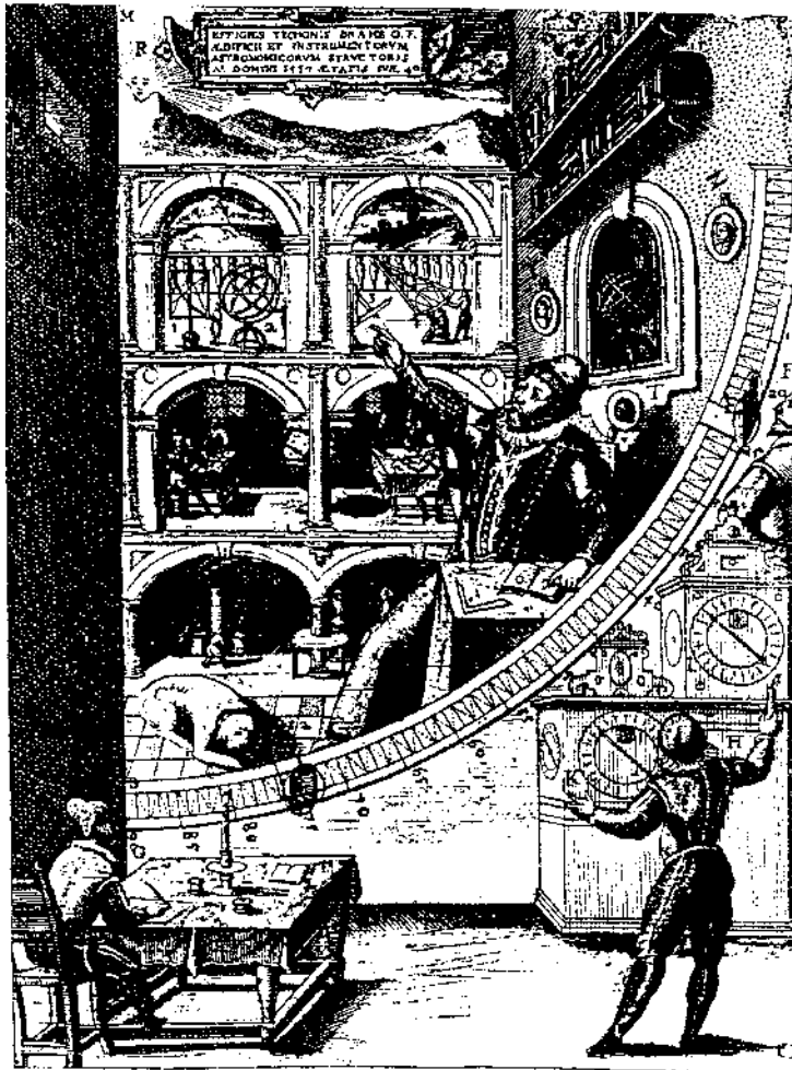
Figure L.5. Tycho Brahe's quadrant was attached to a wall that had on it a painting of Tycho Brahe himself. The engraving shows the observer, presumably Tycho Brahe, someone keeping an eye on clocks so that times of observations could be recorded and someone at a desk noting the readings.
