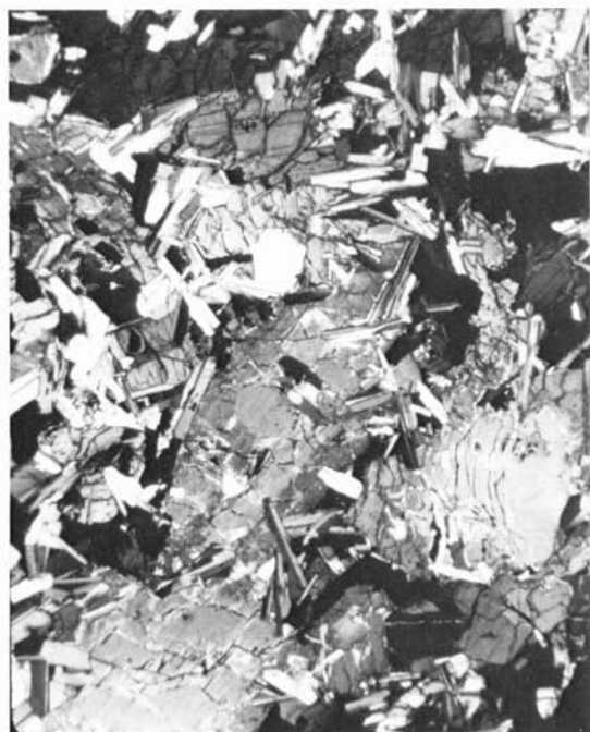
6.28b Apollo 14 high-Al basalt 14053,6. Crossed polarizers 3 \times 4 mm. (Courtesy G. Ryder.)
