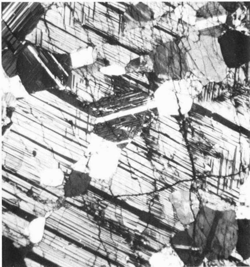
5.4b Monomict cataclastic anorthosite, 15415,29 (Genesis Rock), crossed polarizers, 3 \times 4 mm. (Courtesy G. Ryder.)
