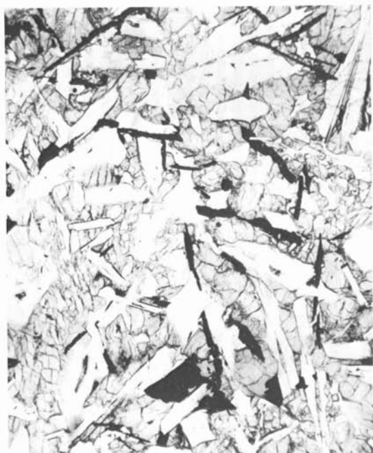
6.27a Apollo 12 aluminous basalt 12038,4. Plane polarized light 4 \times 3 mm. (Courtesy G. Ryder.)
