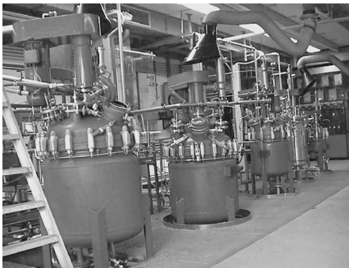
Fig. 7.3. Fermentation plant, University of Regensburg. Partial view, showing two 300 l fermenters and one 130 l fermenter for cultivation of HT.
