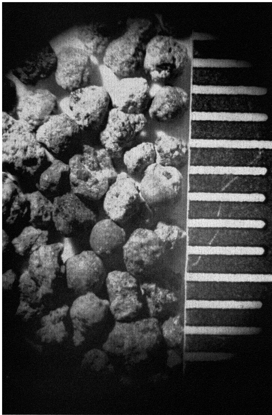
FIG. 1. One particular size fraction ( -10 + 20 sieve meshes) of chondrules separated from the chondrite Bjurböle, with millimeter scale. (Reproduced from Nature 194, 127.)
