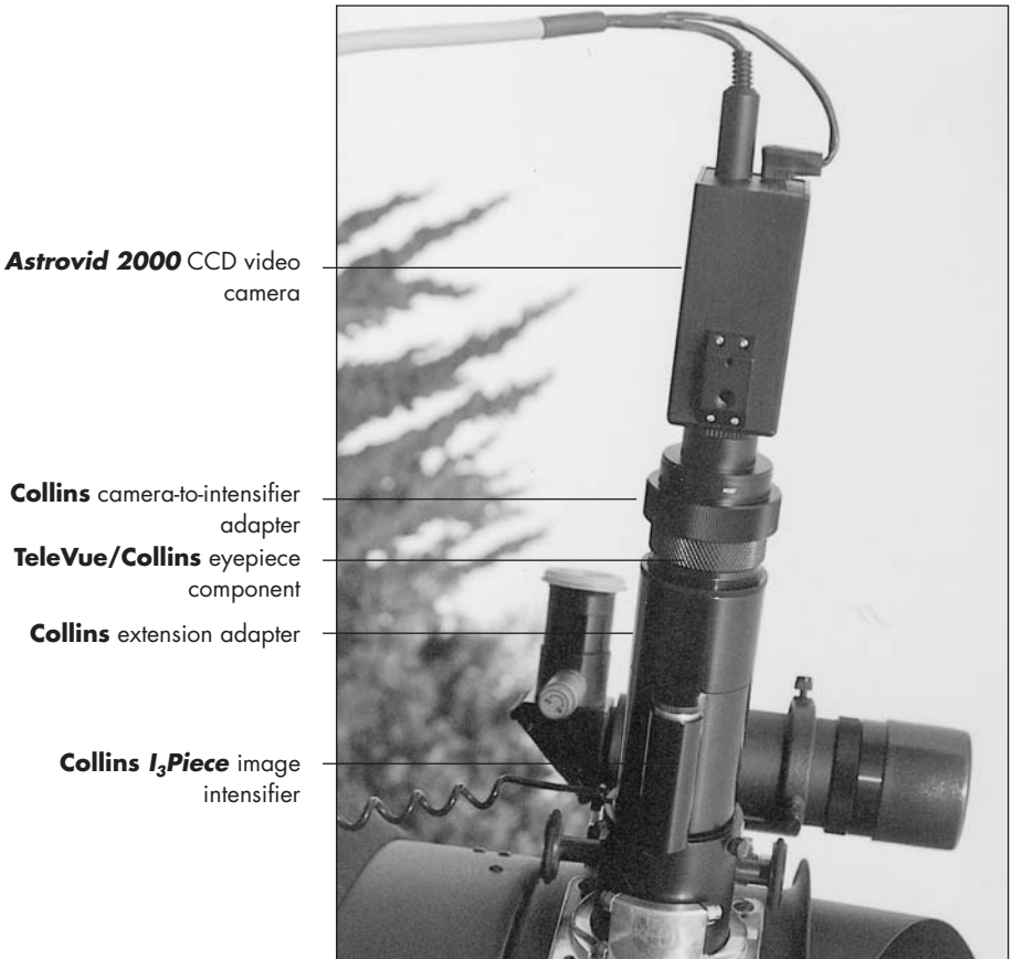
Figure 2.2. Image intensifier and video equipment mounted on the author’s JMI NGT-18 telescope.
