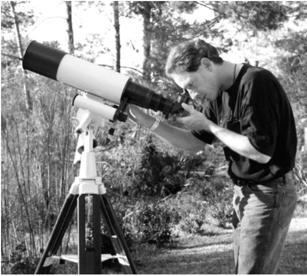
Figure 5.12. The author observes the low sun with the Zeiss SFO white-light filter mounted on a Zeiss APQ 100/640 Apochromat. For safety reasons, all auxiliary optics such as finders should be covered or filtered.
