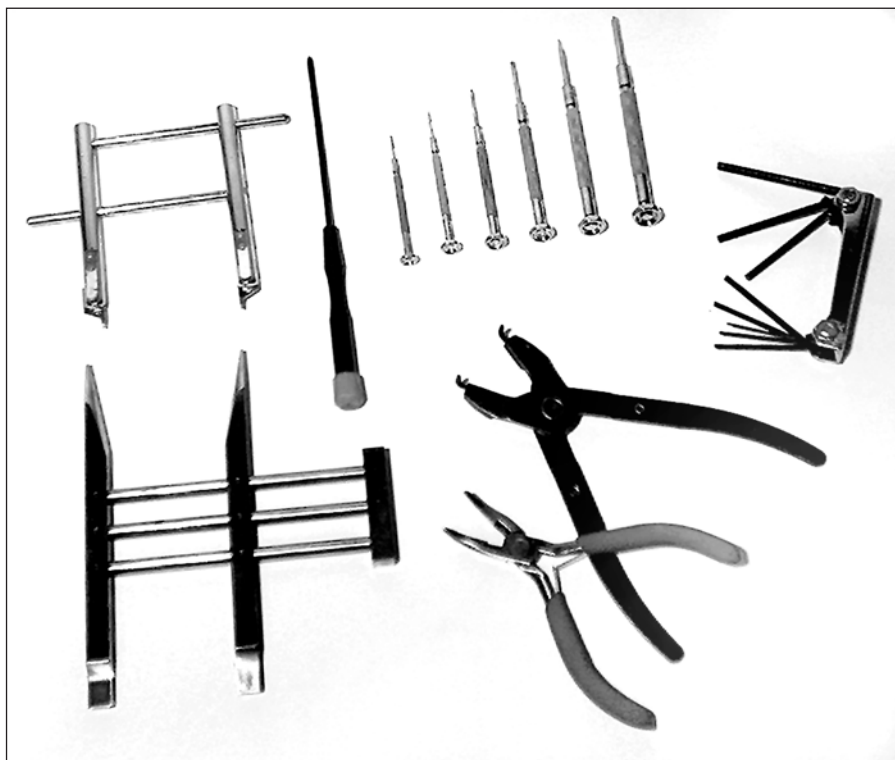
Figure 8.2. A selection of the basic tools needed for disassembling most optical instrument components, including optical spanner wrenches, jeweler's screwdrivers, pliers, and a hex or "Allen" key set for inset-hex head bolts.
