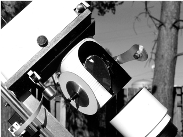
Figure 3.21. The mirror assembly of a portable 70-mm f/11 Polar Siderostat with Solar rate AC drive; the fork-mounted elliptical mirror slews in declination, the entire canister housing slews in right ascension. The projecting silver arm is a dynamical counterbalance. Design and construction: The author.
