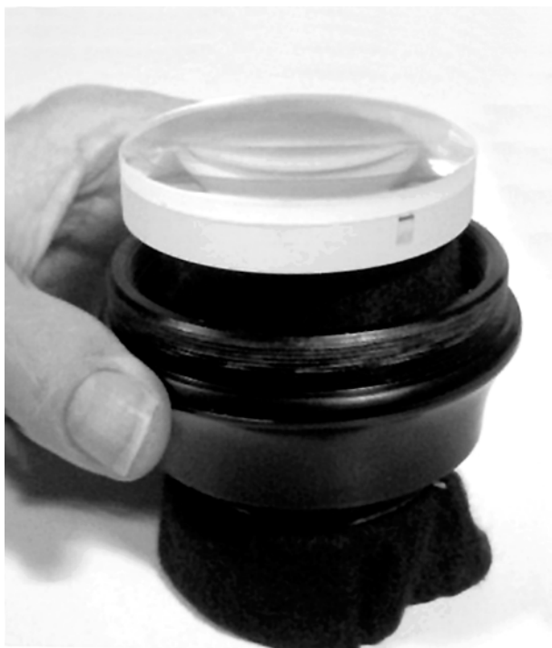
Figure 8.5. An achromat's cell is lowered to remove it from the lens, leaving the lens group accessible on the padded pedestal. Photo: M.D. Pepin.
