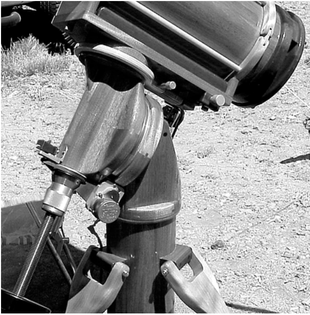
Figure 11.1. Equatorial mounting constructed by J. Hannum and D. Radosevitch using laminated hardwoods. The tube is of similar construction. Photo: Loren Busch.
