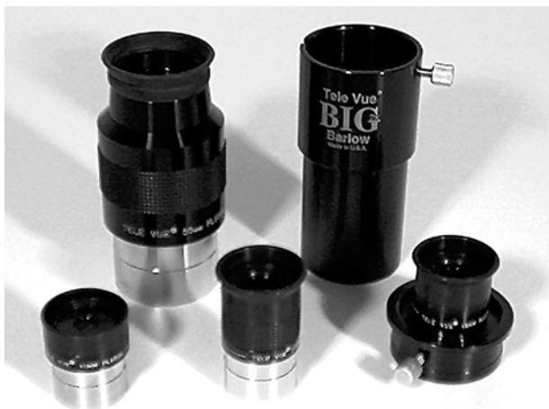
Figure 5.5. The eyepiece selection outlined in the text for the popular 8-inch (20 cm) f/10 SCT adds 2-inch (50.8 mm) format for wide-field. 55 mm, 20 mm, 15 mm, and 11 mm eyepieces, with a 2× Barlow lens, yield a tenfold magnification range, increasing in gradual steps from 1.4° at 36× to 0.14° at 364×.
