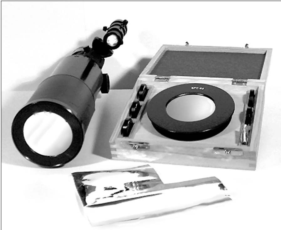
Figure 5.11. Two “white light” solar filter types. Left: Baader Planetarium’s AstroSolar plastic film is mounted in a homemade 100-mm cell on a small refractor, with a sample of the material. The finder is provided with its own small AstroSolar filter, as an aid to acquiring the solar disc. Right: A Carl-Zeiss Jena SFO-80 photo-visual mounted glass filter, in a case with Neutral Density filters. Both types give a view of the Sun in natural color.
