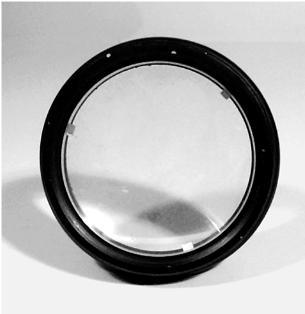
Figure 8.4. View through a small air spaced objective before disassembly. Note the three air-spacing shims on the periphery.
