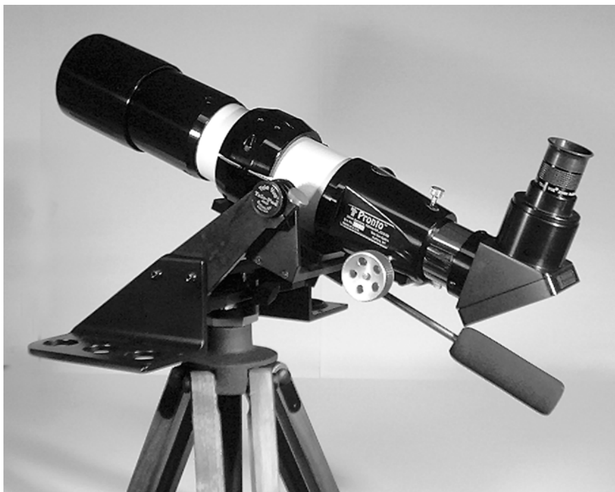
Figure 3.14. This 70-mm aperture semi-Apochromat refractor, a Tele Vue Pronto model, exemplifies the small, fast (f/6.8) new generation of refractors for learners and serious buffs that require a portable glass for air travel and photography. The Gibraltar-model altazimuth mounting is steady and intuitive to use.
