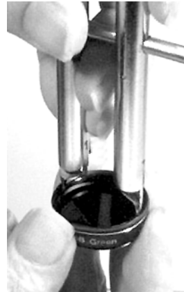
Figure 8.3. Care must be taken not to scratch the glass in removing the retaining ring from a small eyepiece filter cell using an optical spanner wrench. Photo: M.D. Pepin.
