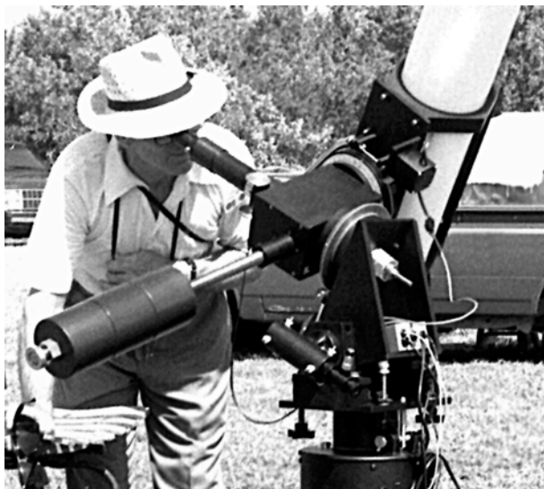
Figure 3.20. An unusual fixed-eyepiece equatorial mounting that uses mirrors to bring the focal plane to a central position on the polar axis. The 6-inch refractor's optical tube is counterweighted to maintain balance, as in a Springfield mount. Design and construction: Thomas Dobbins.
