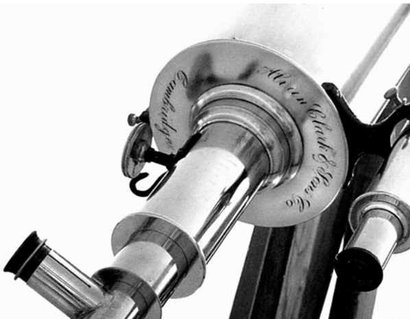
Figure 1.1. Detail of a 6-inch f/15 Clark brass refractor, restored in 1992 by owner Jon Slaton with Steve Sands and Bob Kirschenmann.
