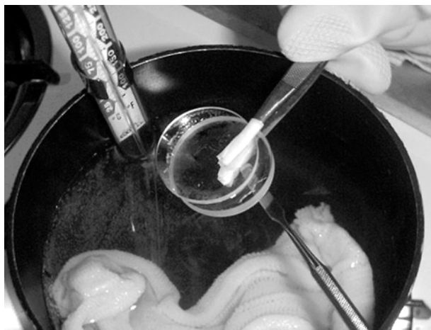
Figure 13.8. The components of the achromat begin to slide apart in the bath at a temperature of 140° F (60° C). Photo: M.D. Pepin.
