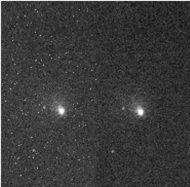
Figure 7.4. Before and after dark subtraction. The image of comet Tempel 1 on the left has not been dark subtracted. The image on the right has. Image credit: Grant Privett.
