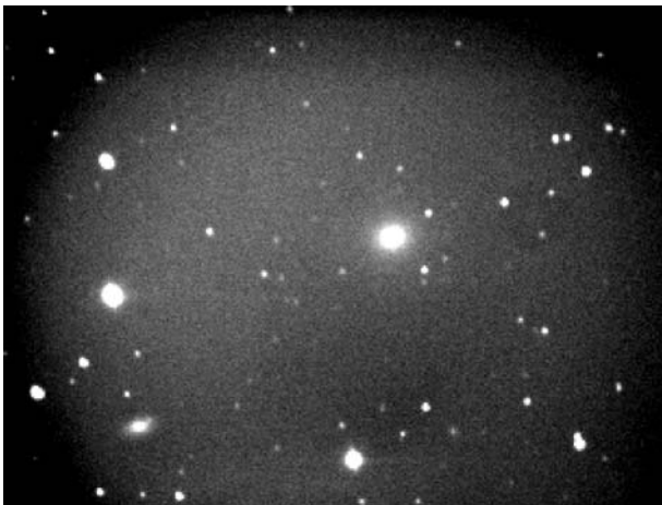
Figure 3.3. An example of image vignetting showing the pronounced darkening at the edges and corners of the image. In this example the fall off from full illumination is quite drastic. In other instances it may be a lot more subtle. In all but the most severe cases flat-fielding can help make the whole image usable. Image credit: Gordon Rogers.
