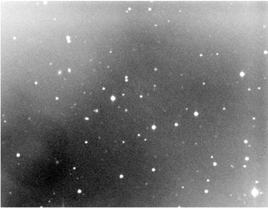
Figure 7.9. Another instance of the unsuccessful removal of a sky gradient. This time the removal of a model has revealed a fault in the flat-fielding – note the large dust doughnut at bottom left. Image credit: Grant Privett.
