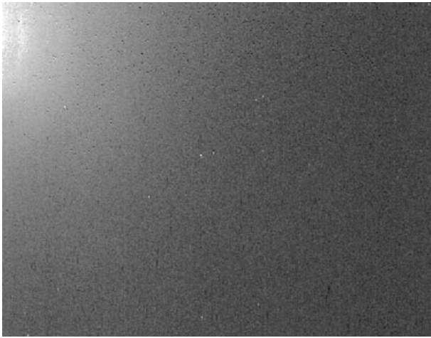
Figure 7.2. A typical dark frame for a CCD sensor made in 2003. Note the brighter upper left corner where a signal caused by the on-chip amplifier can be seen. This will be easily removed from images by dark subtraction, due to its small amplitude. In the remainder of the image there are a small number of hot pixels. Overall, the noise from the on-chip electronics and thermal sources is considerably reduced compared to its 1994 predecessor. Image credit: Grant Privett.
