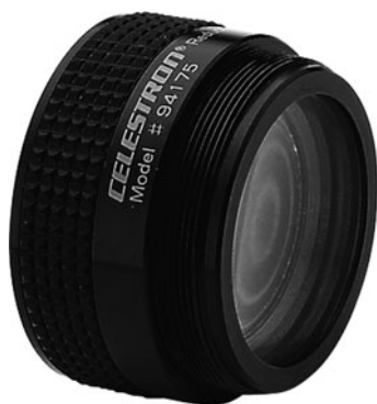
Figure 1.4. Reducer-correctors are useful for shortening the focal length of an SCT while also flattening the field. This makes such telescopes much better tools for observing deep sky objects such as open clusters that have a large angular diameter. (Photo courtesy of Celestron.)
