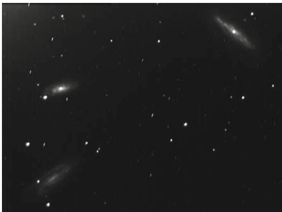
Fig. 4.10. Sky frame of the subject shows some amplifier glow and several hot pixels (NGC 7582-90-99).
