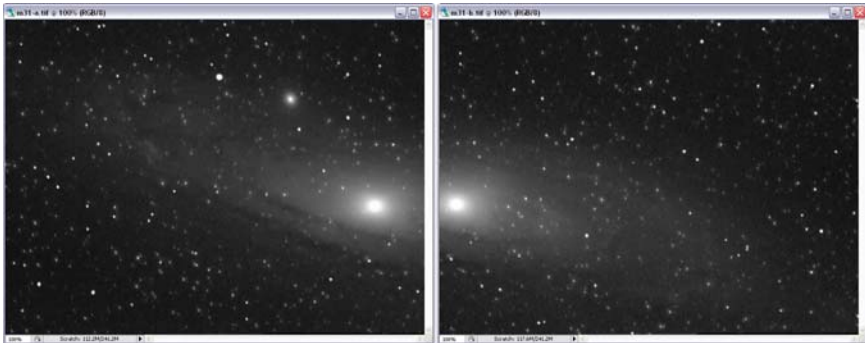
Fig. 6.66. Two separate fields showing each half of the galaxy Messier 31 with an overlap of about 15%. Imaged through a 300-mm lens with a GSTAR-EX camera.
