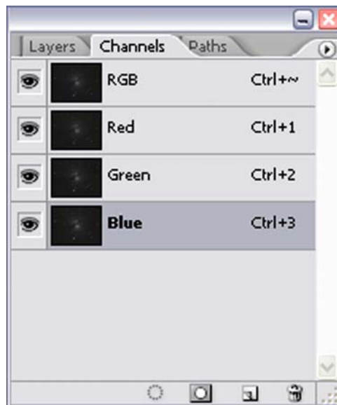
Fig. 6.33. All the “eyes” are on, but only the blue channel is active ( highlighted ).
