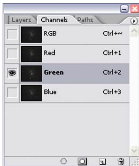
Fig. 6.30. Pasting the green image into the green channel of the red image.
