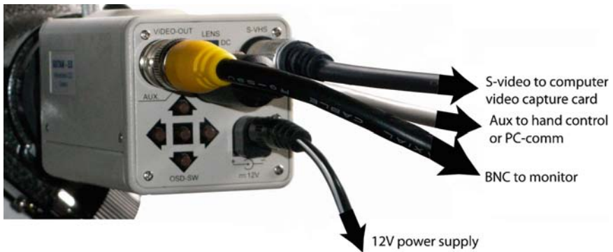
Fig. 2.13. Back panel connections of the GSTAR-EX camera.
