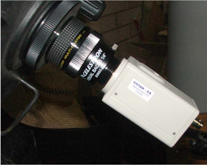
Fig. 4.2. A C11 Schmidt Cassegrain fitted with a Meade f/3.3 focal reducer via camera adaptors. Because of limited focus travel, this configuration does not allow most common filter selectors to be fitted into the optical train. Courtesy of Mike Holliday.
