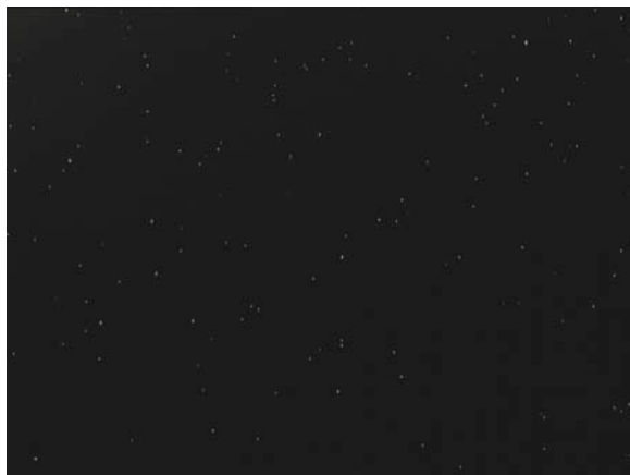
Fig. 4.11. Dark frame of the same recording time and settings as the sky frame.
