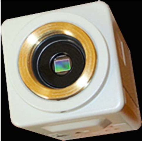
Fig. 1.2. At the heart of all modern digital cameras, the CCD collects photons and converts them into an electrical charge to create an image.
