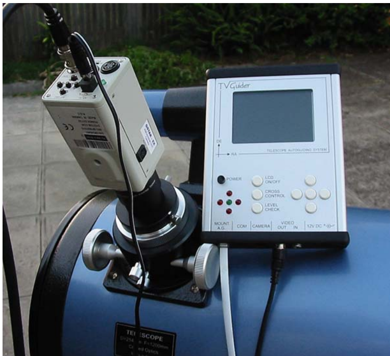
Fig. 7.11. The nicely constructed and affordable TV Guider system developed by Martin Myslivec of the Czech Republic, interfaced to the autoguider port of an EQ6 equatorial mount.
