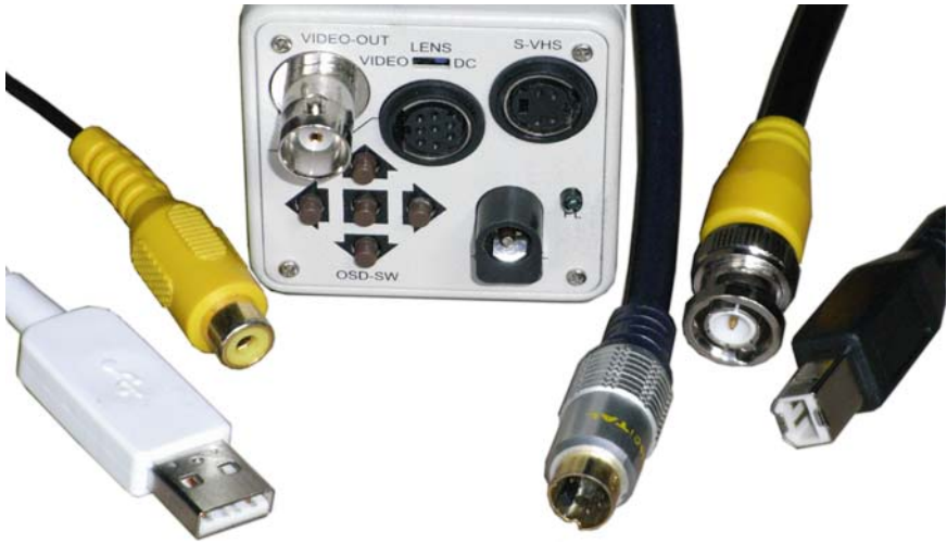
Fig. 2.14. Various camera connector interfaces including composite, S-video, and digital.
