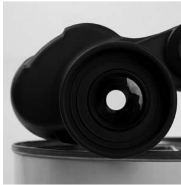
Figure 1.3. The exit pupil is a small disc of light that can be seen behind the eyepiece. Its size depends on the magnification and the entry pupil diameter
