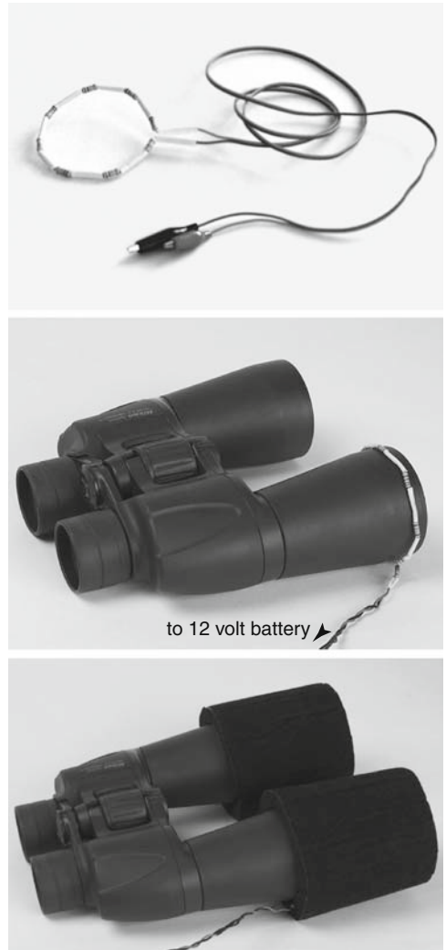
Figure 1.12. Top: The warmer is made from resistors that are connected in a series. All metal parts should be kept well isolated, so that you do not create a short circuit. Middle: The warmer is attached to the casing as close as possible to the optics. Bottom: The most effective is the combination of the warmer and protective tube
