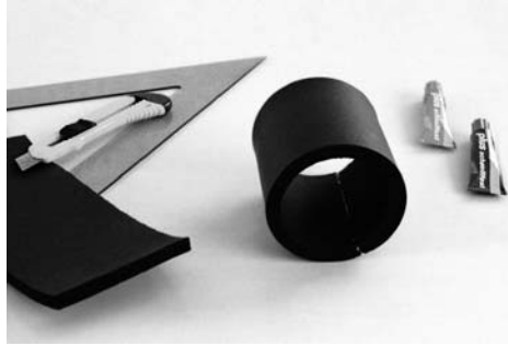
Figure 1.11. The protective tube for the objective of the binoculars, made from rubber foam
