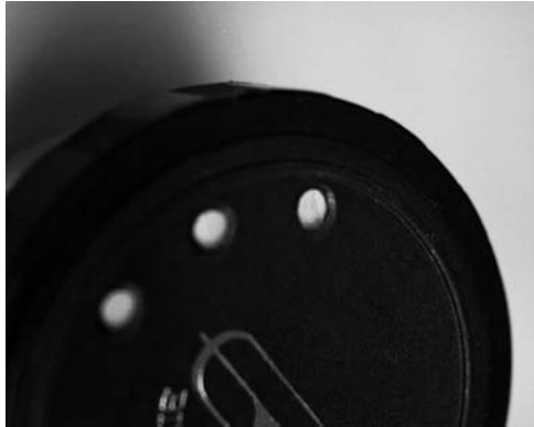
Figure 1.10. If the temperature in the room in which you keep your binoculars oscillates, the optics under the protective caps will often mist up. In order to prevent this from happening, make a few holes in the protective cap and cover it with a net plastic fabric (such as Gore-Tex™ or printing foil). Dust will not gather on the lenses, but the moisture will evaporate during the temperature oscillations
