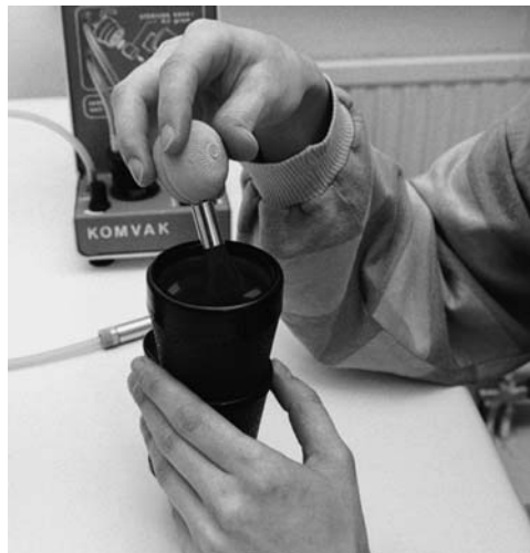
Figure 1.9. When cleaning with a brush it is very important that the dust particle stays in contact with the glass surface for the shortest time possible. Gently touch the surface with the brush and rotate it. This demands a steady hand and some practice
