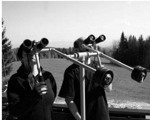
Figure 1.7. This tripod, which consists of water pipes, can easily be made by one person. Many different plans for constructing a tripod can be found on the Internet
