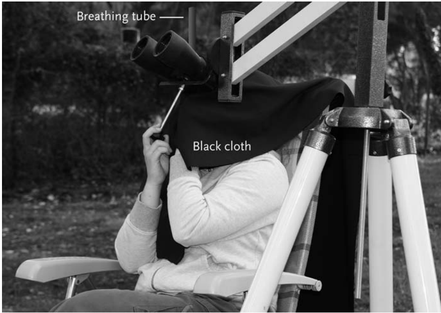
Figure 10.17 Here is the best way to observe such elusive objects as the galaxy NGC 7331 . A black cloth over your head and binocular eyepieces prevent peripheral light from disturbing your observations. Only in complete darkness can your eyes fully adapt to night vision. A breathing tube is indispensable for preventing dew forming on the eyepieces, which would be caused by your exhaling. In fact, all celestial objects should be observed like this. But if you do this make sure you tell your neighbors what you are going to do first; otherwise, they just might think you have lost it
