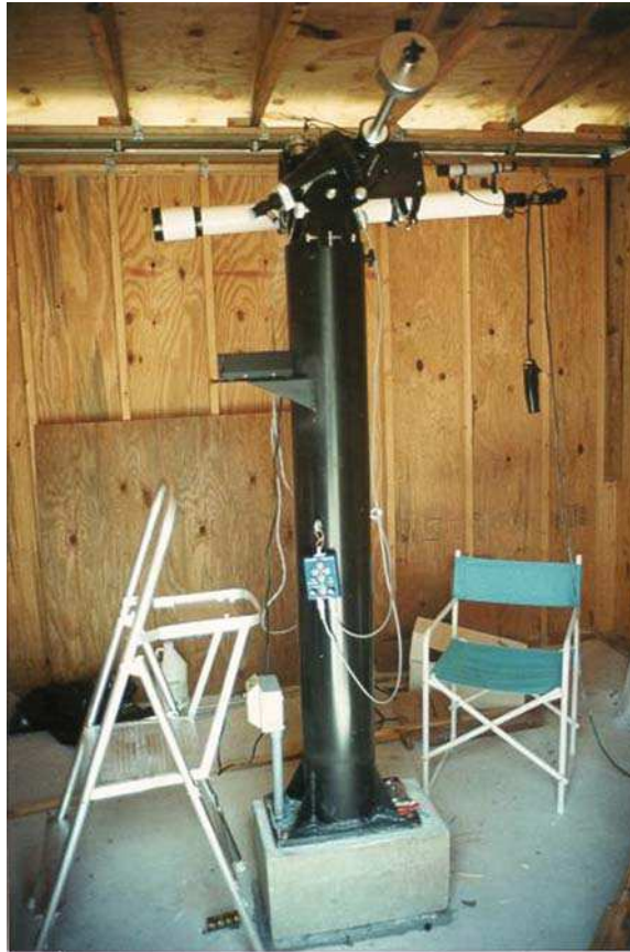
Figure 2.1. Mid-construction test: Refractor fits under closed roof when rotated completely horizontal. If calculations had been incorrect, the pier or cement base pedestal would have to be shortened. (From the collection of John Hicks).
