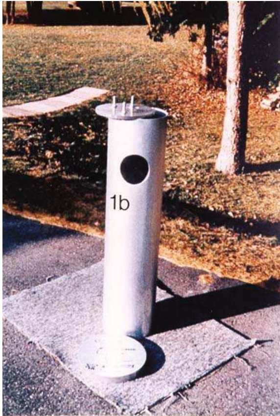
Figure 4.2. Typical Aluminum or Steel Pier top showing end-plates: - the top plate with bolts protruding to accept the telescope mount, the bottom plate with pre-drilled holes to fit bolts from cement footing underneath. Note the access-holes sawn into the tube required for tightening up the bolts from inside. Both top and bottom plates were drilled and tapped to take large threaded bolts. The access holes serve another purpose also; - the tube can be filled with sand from this point to dampen any vibration in the pier. (Photo by John Hicks).
