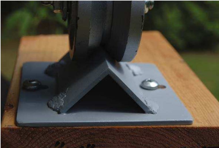
Figure 8.1. Photo - V-Groove caster on section of inverted angle resting on double 2" x 6" plate. (Photo by John Hicks).
