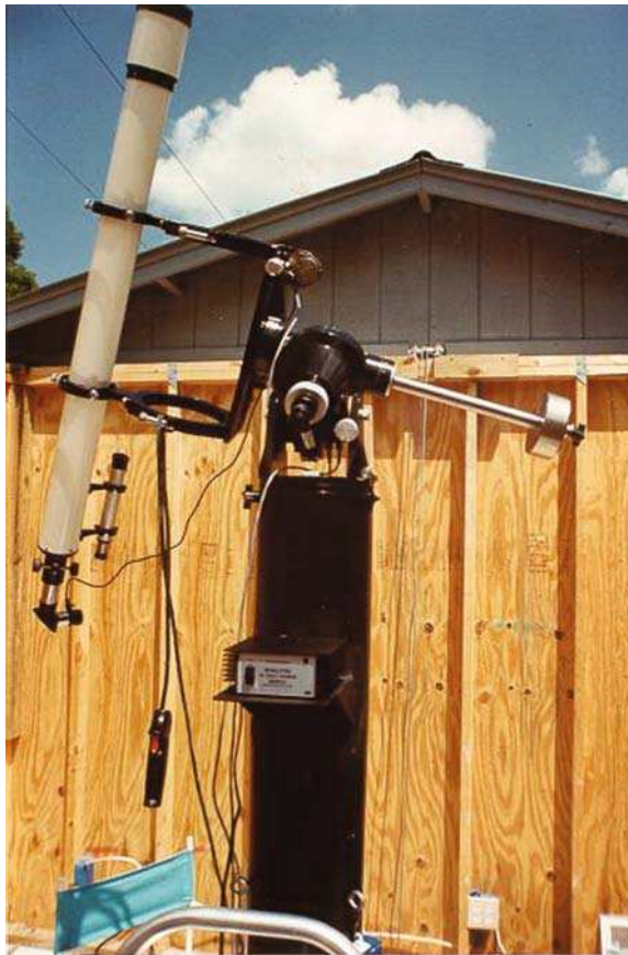
Figure 6.12. Photo – Guidscope on Mount intended for large refractor awaits final construction. At this point the cradle rings justify calculating the horizontal rest position of the final telescope assembly. (From the collection of John Hicks).
