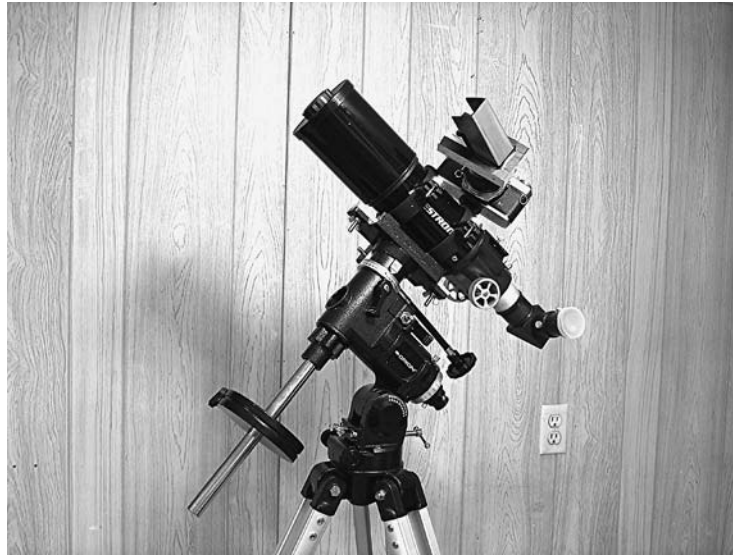
Figure 16.3. The spectrograph mounted on an 80-mm f/5 refractor.
