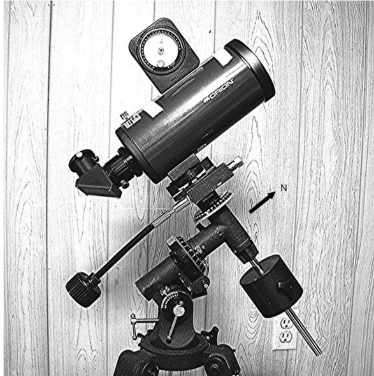
Figure 3.8. Adjusting the inclination of the polar axis.
