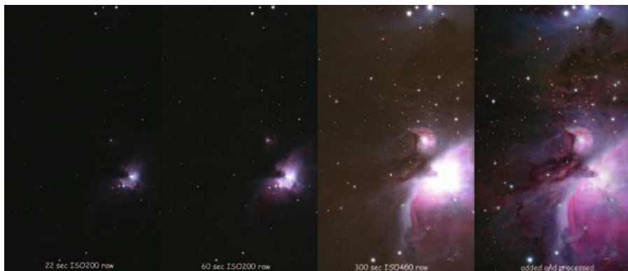
Figure 5.10. Adding exposures of different lengths preserves the detail that would otherwise be burnt out in the brightest areas. This image comprises crops of 3 raws from the left to right that have been added in the following way: 2 \times 20 sec, 8 \times 60 sec and 26 \times 5 min. The final combined result is shown in the image crop at right. The telescope was the 4-inch TMB refractor with reducer at f/5 .
