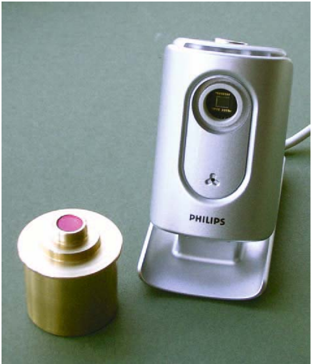
Figure 3.2. Toucam Pro II with 1.25-inch adapter. Note that the infrared block filter from the rear of the original lens has been refitted into the adapter.
