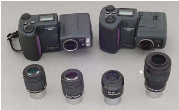
Figure 2.7. The older Nikon Coolpix 990/995/(4500 not shown) digital cameras are excellent afocal photography cameras when used with eyepieces having 28mm camera threads. Eyepieces from left to right: ScopeTronix 14mm & 18mm, William Optics 24mm and ScopeTronix 40mm.
