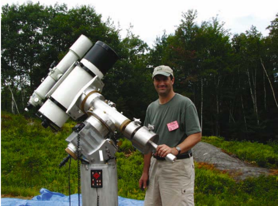
Figure 8.7. Brian Lula and portable imaging setup. Reinforcing Brian's opinion about mount rigidity for CCD imaging is his design of a portable German equatorial mount for scopes up to 16-inch diameter with long focal lengths. It is shown here at the Stellafane Amateur Telescope Making Conference.
