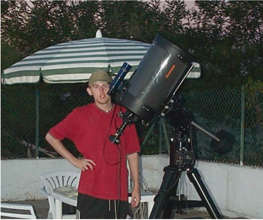
Figure 7.2. The author and his 28cm scope ready for action, with the imaging PC located close by. At the rear of the scope, the ATK-1HS is seen attached.
