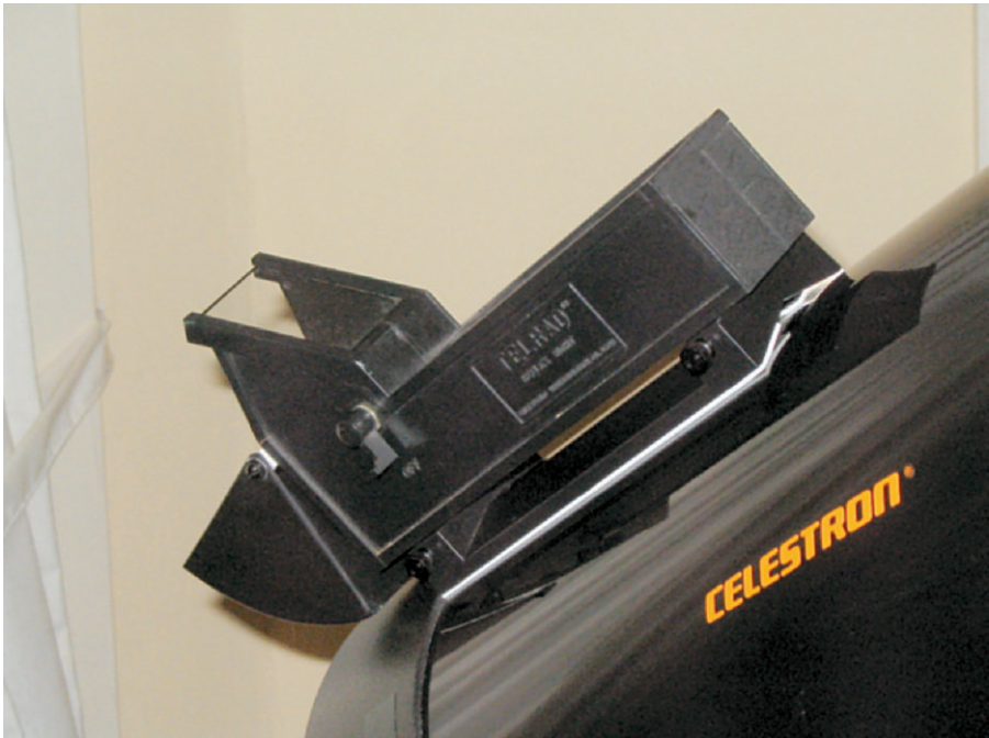
Plate 10. Steve Kufeld's ingenious TELRAD aiming device.
