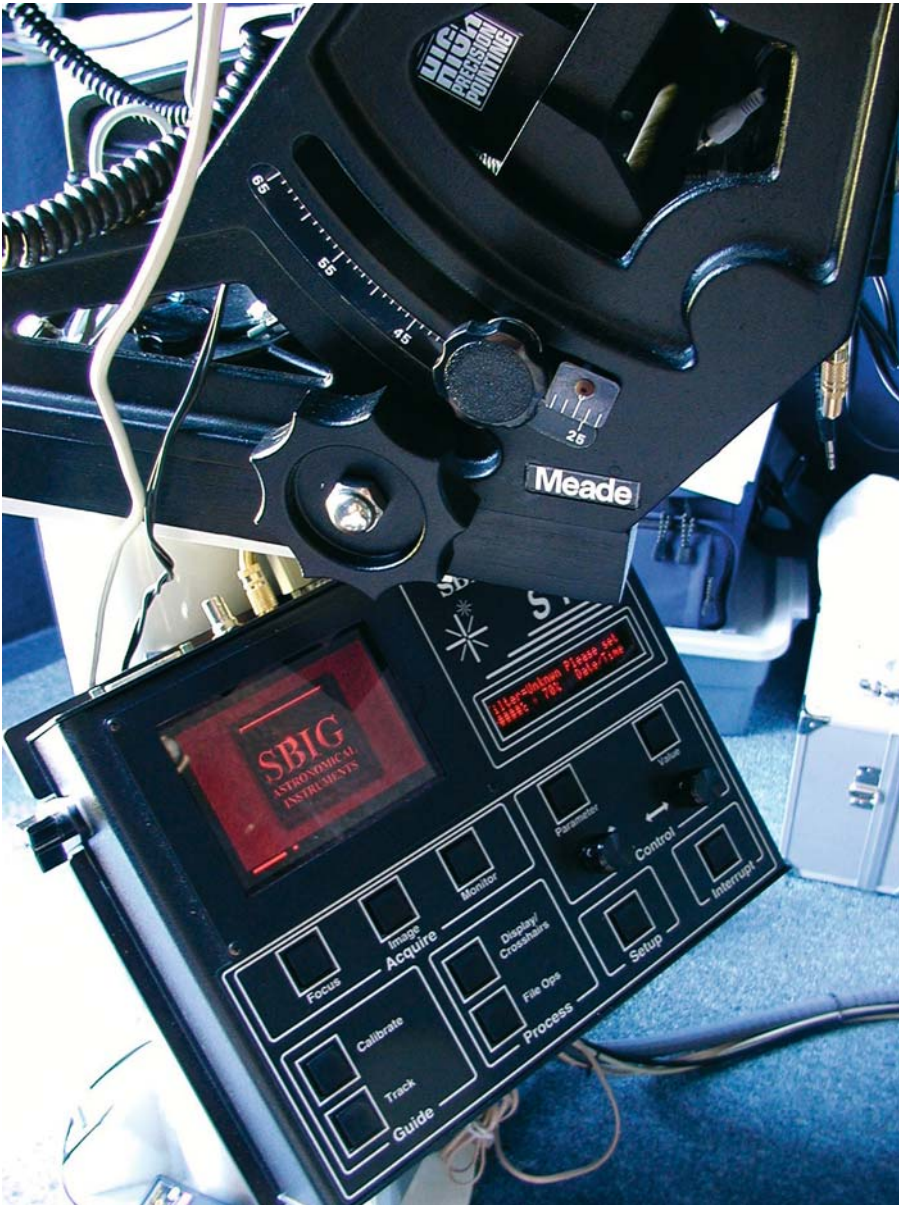
Figure 2.24. STV Deluxe video output can be viewed on built-in 5-in. LCD screen or on a television monitor via video cable. (Used with permission, Santa Barbara Instruments Group).
