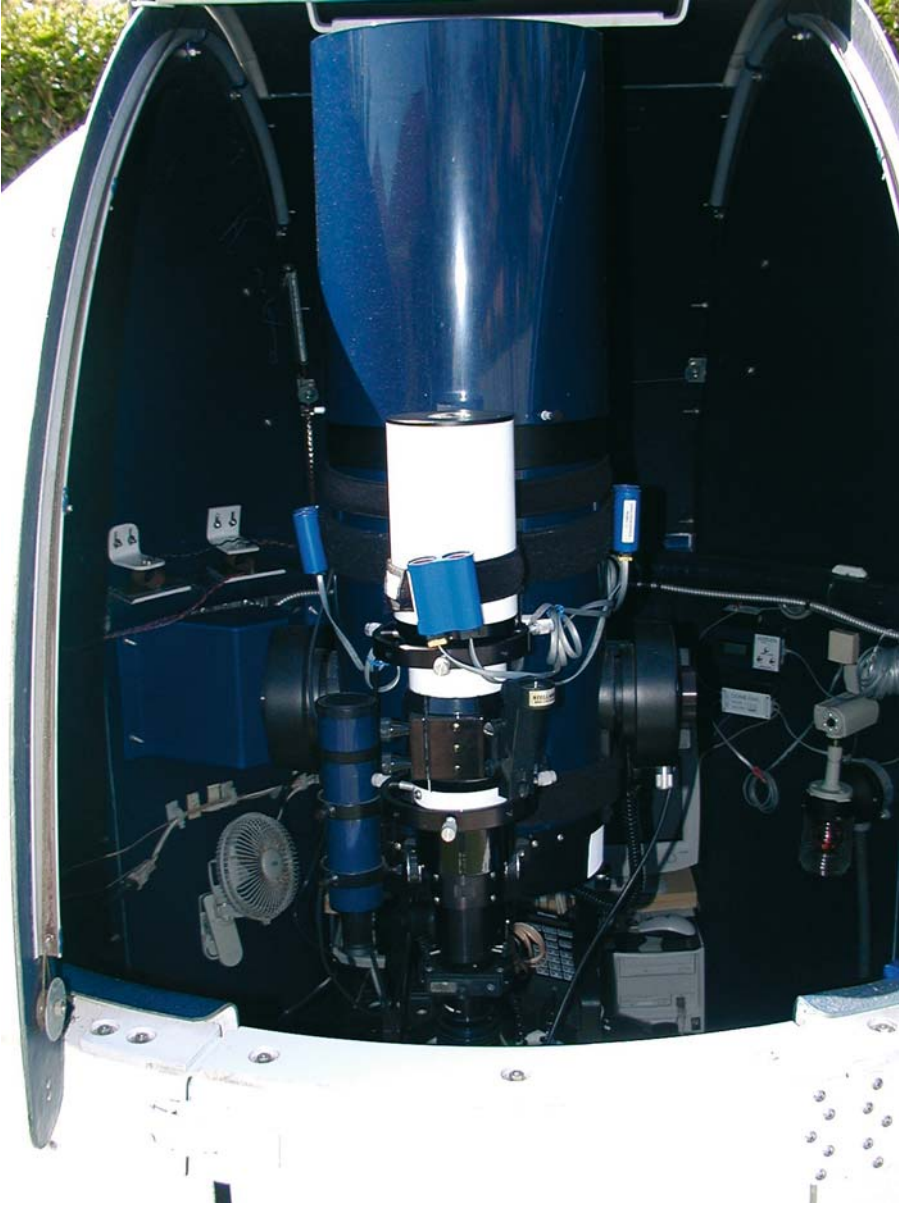
Figure 2.2. Piggybacked Stellarvue Nighthawk and Meade LX200. The large blue metal dew shield on the LX200 almost extends out of the observatory. The blue attachments are infrared detectors, part of the Dome-Works™ system. A small Meade guide scope is to the left of the refractor. Black heating straps circle the dew shields of both telescopes and are part of the Kendrick Dew Heater system. (Used with permission, Stellarvue® Telescopes, Meade Instruments, Technical Innovations, and Kendrick Astro Instruments, respectively.)
