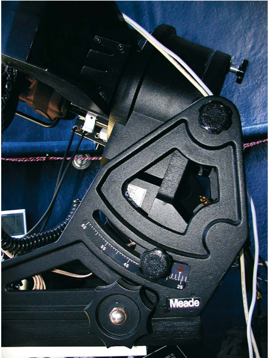
Figure 2.6. LX200 drive base attached to Superwedge and Astro Pier™. Take note of the angle at which the drive base is attached to the wedge tilt-plate ( 26^\circ for my latitude).
