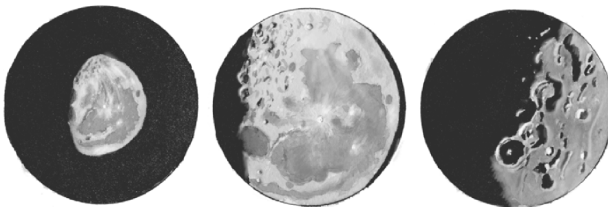
Fig. 4.3. As a telescope's magnification increases, the actual amount of the sky seen decreases (making low powers preferred for many types of observing, such as sweeping for the Herschel objects). Shown here are three stylized sketches of the Moon at low, medium, and high magnifications. While the image gets bigger at higher powers, less and less of it can be fitted within the eyepiece's field of view.
