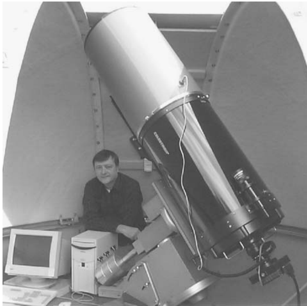
Figure 10.10. Tom Boles with his oldest Paramount GT1100/Celestron 14 system, inside a dome at Northampton. This system is still used during windy conditions from his Suffolk observatory, when the run-off observatory telescopes are too exposed to wind vibration. Image: Tom Boles.
