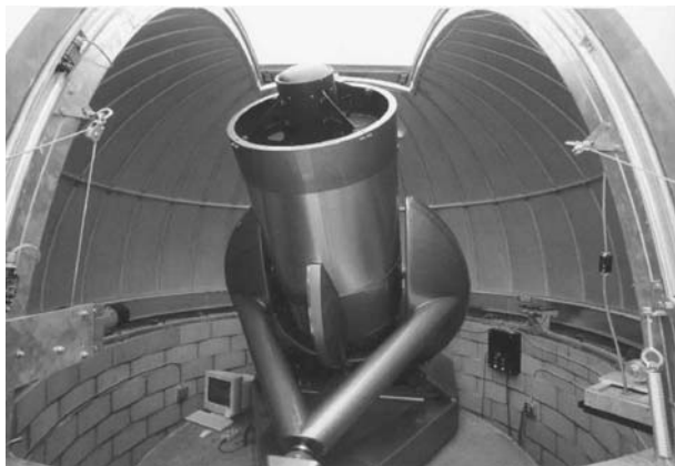
Figure 10.2. The massive Tenagra II 0.81-m f/7 Ritchey-Cretien of Michael Schwartz: the largest amateur telescope used for supernova discoveries. Image: Michael Schwartz.
