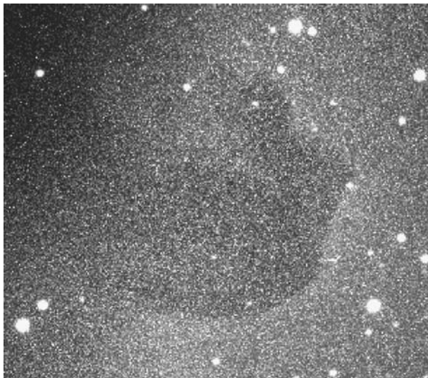
Figure 7.2. The Horse-head Nebula in Orion taken with a Celestron 14 at f/7.7 , a 180-second exposure, and an SBIG ST9XE CCD, but with no dark frame subtracted. Image by the author.
