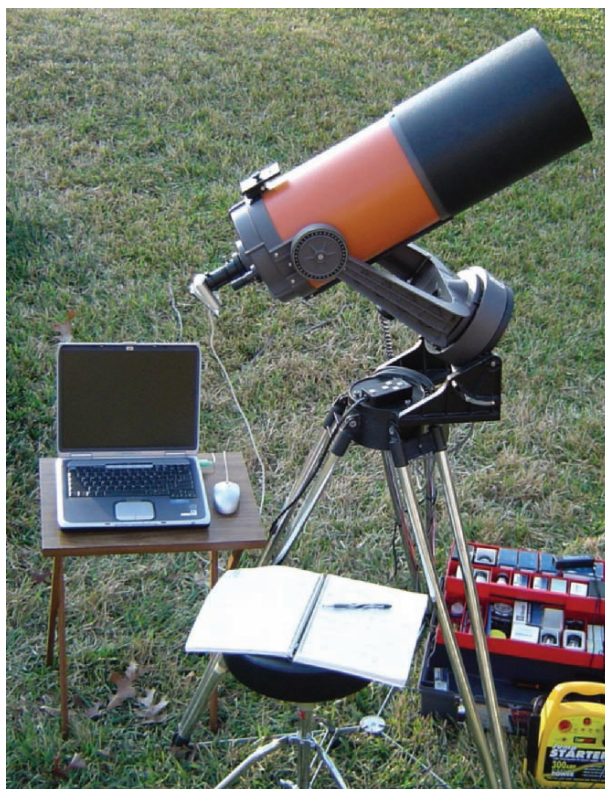
Fig. 9.11. The authors webcam imaging setup, including webcam, laptop computer, telescope, portable electric power source for the telescope clock drive, and the all important logbook for recording the imaging data. (Credit: John W. McNally).
