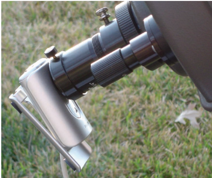
Fig. 9.10. A webcam mounted into the eyepiece holder of a telescope ready for imaging. A 2x barlow lens is inserted between the telescope and the camera to increase the focal length to f/20 . (Credit: John W. McAnally).
