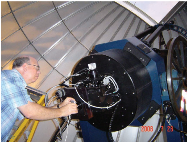
Fig. 9.12. The webcam can be used in any size telescope. Here the author installs his webcam into the eyepiece port of a 2-ton, 24-in. (0.61 m) professional classic cassegrain. (Credit: Trudy LeDoux/the Central Texas Astronomical Society).
