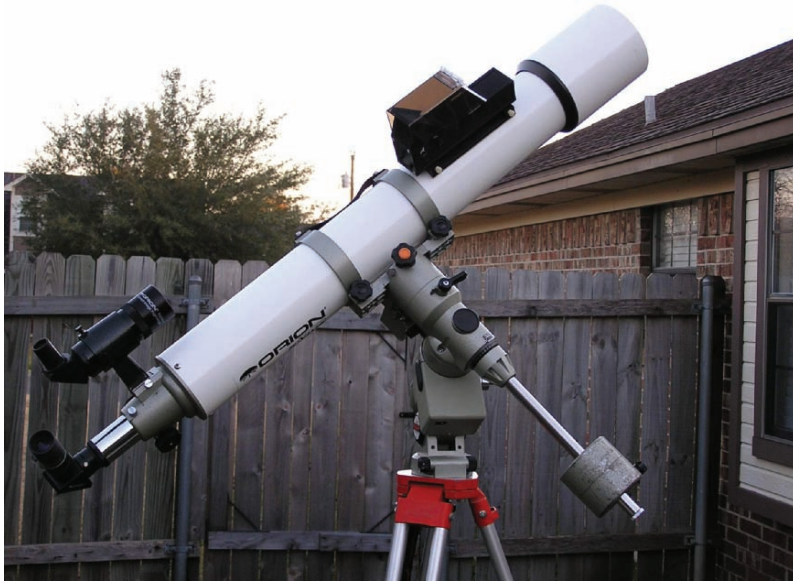
Fig. 7.1. A typical refracting telescope on a German-equatorial mount. (Credit: Brady Richardson).
