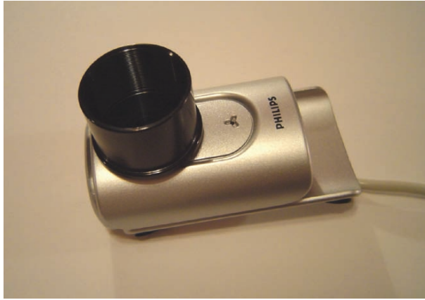
Fig. 9.9. A Phillips ToU Cam Pro webcam, used to capture images of the moon and planets. (Credit: John W. McAnally).
