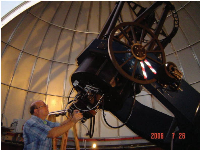
Fig. 7.3. The author behind a 24-in. (0.61 m) classic cassegrain reflecting telescope, a 2-ton professional instrument in a professional observatory owned by an amateur organization. (Credit: Trudy LeDoux/the Central Texas Astronomical Society).
