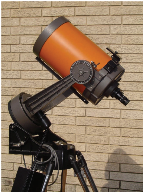
Fig. 7.4. An 8-in. (203 mm) Schmidt-cassegrain reflecting telescope on a fork-equatorial mount and tripod. (Credit: John W. McAnally).
