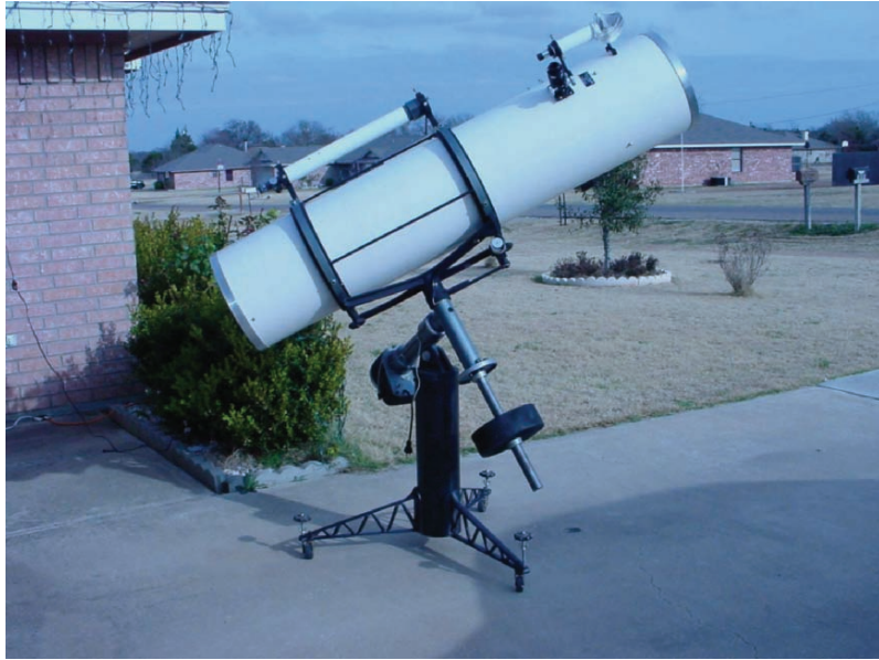
Fig. 7.2. A 12-in. (305mm) Newtonian reflecting telescope on a German-equatorial mount. (Credit: Dave Eisfeldt/the Central Texas Astronomical Society).
