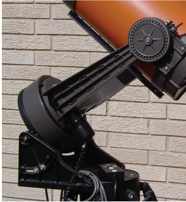
Fig. 7.8. A close up of a fork-equatorial mount, complete with setting circles on both the polar and declination axis. Electric clock-drive motors are concealed in the large circular base. (Credit: John W. McAnally).
