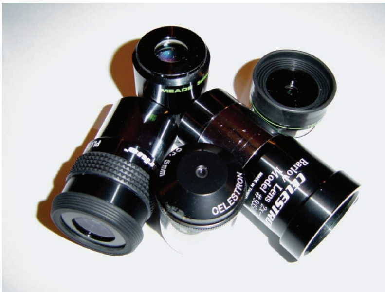
Fig. 7.5. An assortment of eyepieces, both orthoscopic and plössl, and a \times 2 barlow lens. (Credit: John W. McAnally).
