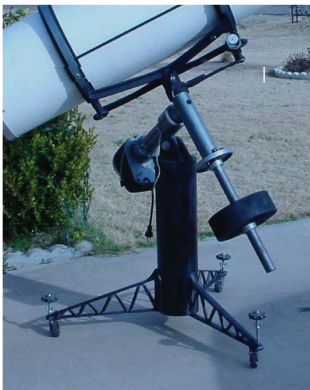
Fig. 7.7. A strong German-equatorial mount on a portable pier, made to carry a heavy telescope. The counter weight shown weighs over 50 lbs. (Credit: Dave Eisfeldt/the Central Texas Astronomical Society).
