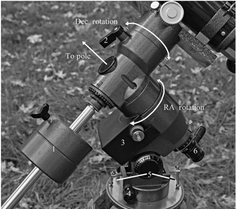
Figure 3.16 The German equatorial mount. (1) Counterweight and counterweight shaft. The counterweight is used to balance the telescope, so that it is easy to move (either by hand or with the drive), and so that it stays in place once the movement is done. To use it, you loosen the bolt visible on the top of it, and slide the counterweight on the shaft to find the proper, balanced point, and then tighten again. (2) Declination lock lever (the RA lever is on the other side of the mount, so not visible in the photo). When the levers are unlocked, it is easy to move a well-balanced scope close to the observing target by simply pushing and pulling by hand. Once close, you can lock the levers, and make final adjustments with the slow-motion hand controls, or with the electronic hand controller. (3) Right ascension motor housing. When this motor is running, the mount's motion matches that of the turning of the Earth, keeping objects centered in the eyepiece. (4) Azimuth adjustment knobs. (5) Altitude adjustment bolts. The azimuth and altitude adjusters are used only to align the mount with the celestial pole; they are not meant to help you in aiming the telescope. (6) Polar alignment scope. This is a small telescope that is mounted right inside the mount, and is used to help you get accurate alignment with the pole.
