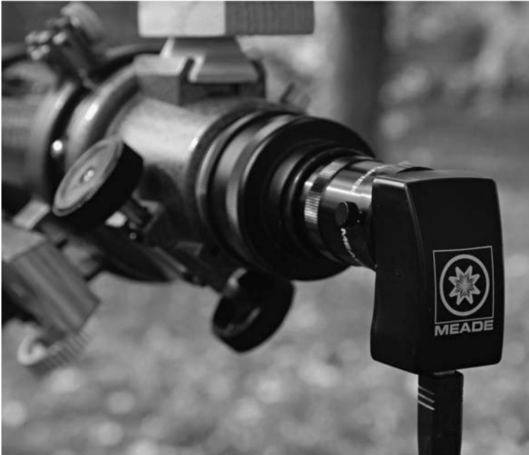
Figure 3.31 A small digital astrocamera, made to photograph bright objects like the Moon and planets. It requires a computer at the telescope.
