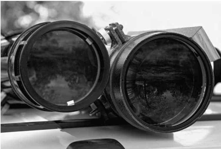
Figure 3.5 If all other things were equal, the telescope on the right, with an aperture of 100 mm (about 4 inches) should not only produce 56% brighter images, but also sharper images, than the 80mm scope on the left.
