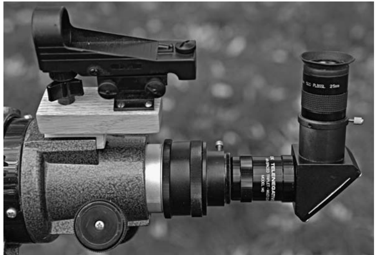
Figure 3.21 In the small area near the focuser of this scope you can see many of the items described in this section: an eyepiece, diagonal, Barlow lens, and finder.
