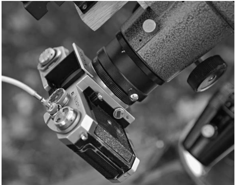
Figure 3.30 An old SLR film camera attached with an adapter directly to a telescope’s focuser, for prime-focus astrophotography.
