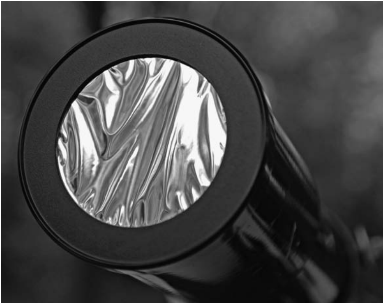
Figure 4.5 A solar filter in its proper place: in front of the objective lens or mirror of a telescope. This one is made of mylar.
