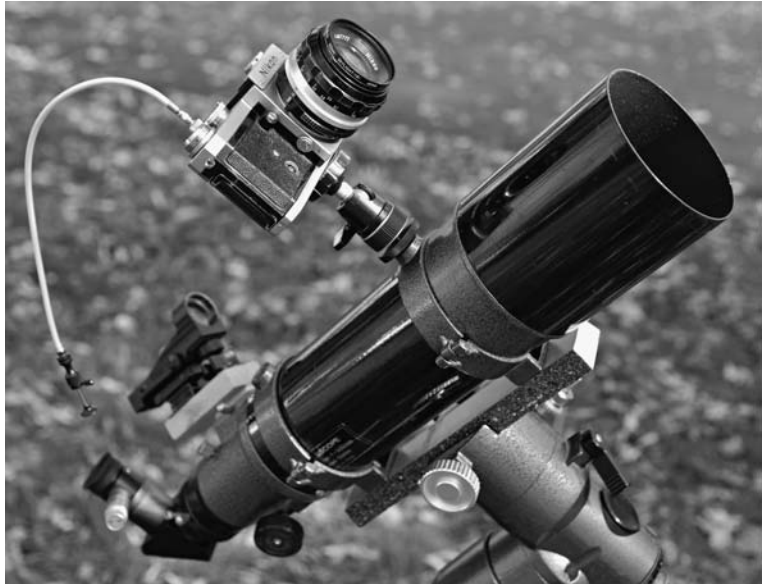
Figure 3.29 A telescope set up for “piggy-back” astrophotography; the cable release on the camera, and the illuminated reticle eyepiece seen in the telescope’s focuser, are almost essential for sharp, guided photos.
