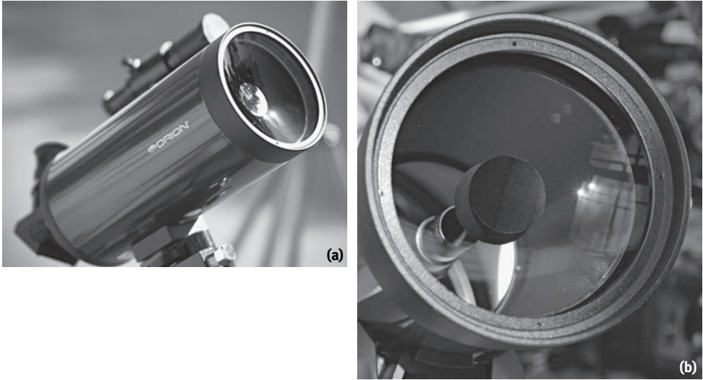
Figure 3.13 (a) Because of the complex path and four curved surfaces of a Mak, this short (less than 12 inch) tube is able to house a 102-mm (4-inch) aperture scope with a focal length of 1300 mm. (b) The mechanics of a Mak: visible here are the meniscus lens/corrector plate, the secondary mirror attached to the plate's center, the primary mirror, and the focuser housing coming through the primary's center.
