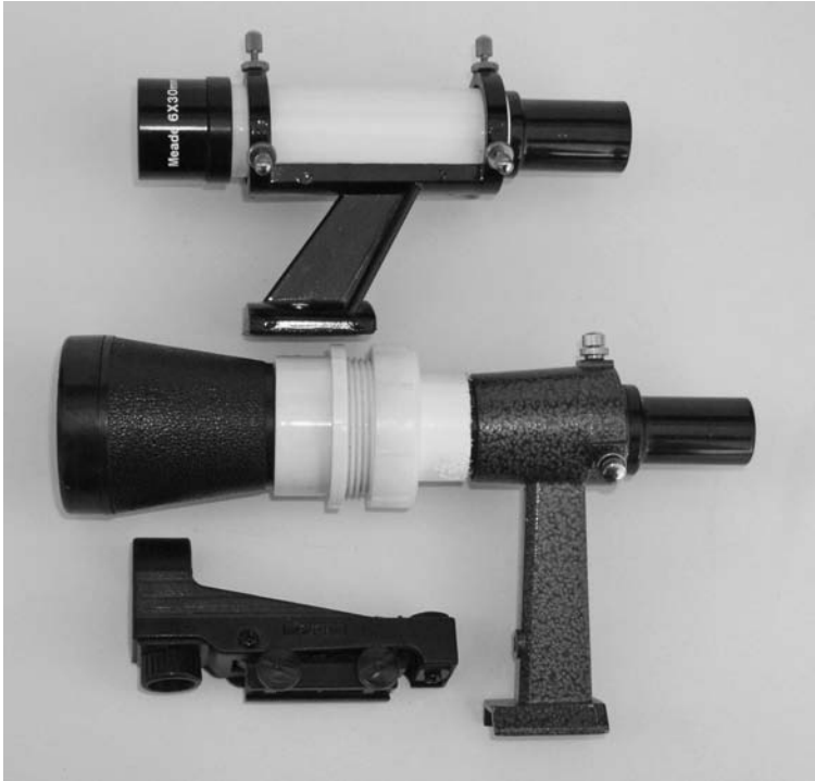
Figure 3.26 Three quite different finders. Top: a 6 x 30 finder scope that comes as a standard on many smaller scopes; middle: a finder that started out as a 6 x 30, but which has been modified with the objective end of a broken pair of binoculars into an approximately 8 x 50 finder scope; bottom: a “red-dot” or unit power finder.
