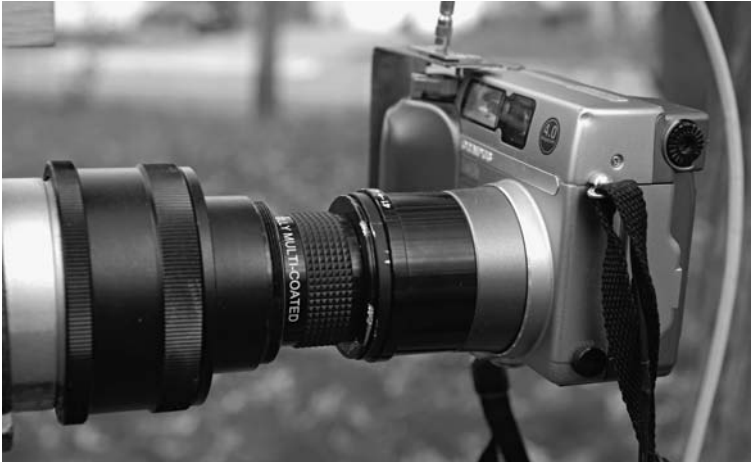
Figure 3.28 Afocal astrophotography: A point-and-shoot digital camera attached, with a screw-on adapter, to an eyepiece inserted into a telescope's focuser.
