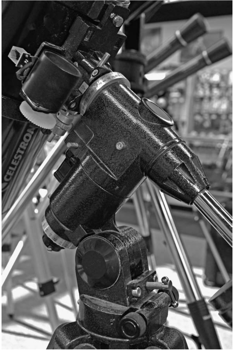
Figure 3.18 The mid-sized CG-4 (or EQ-3) mount.
