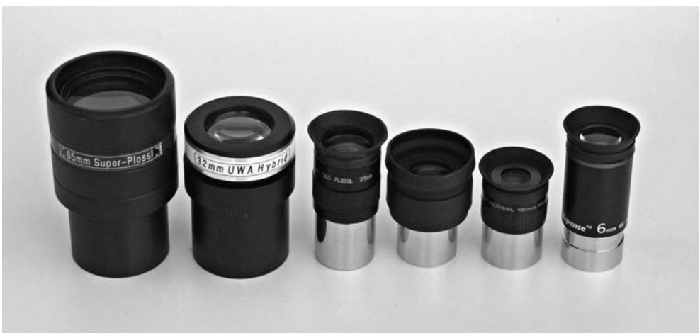
Figure 3.22 Eyepieces come in a wide range of size, focal length, and quality. Here are two 2-inch (on the left) and four 1.25-inch good-quality eyepieces that would provide magnifications, in a telescope with a focal length of 1000mm, of, from left to right, 15.4×, 31×, 40×, 59×, 67×, and 167×.
