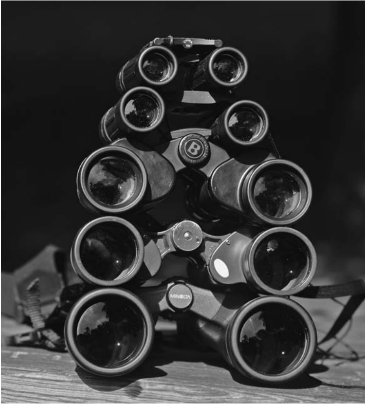
Figure 2.4 Comparing binoculars: From top to bottom, here are the pairs of numbers that describe the magnifications and apertures of each of these pairs of binoculars: 8 x 20, 10 x 25, 7 x 35, 10 x 42, and 10 x 50. The top two are not appropriate for astronomy: they are poorly made, with low-quality roof prisms, and each pair has an exit pupil of only 2.5 mm. The bottom three are much better choices: they all have good- to excellent-quality porro prisms; they have larger objective lenses; the exit pupils are at least 4.2 mm; and those circles between the lenses are covering threaded tripod-mounting holes. Note also the reflections off the objectives. The middle pair of the bottom three has the fewest, and this is a sign of excellent multi-coatings, which is also a likely pointer to overall quality. They are, in fact, the most expensive pair of the five.
