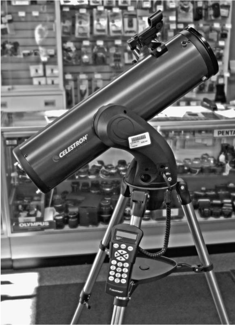
Figure 3.20 Perhaps the largest-aperture go-to telescope within this guide's price range: a 130 mm (5.1 inch) Newtonian reflector with a focal length of 650 mm (for a focal ratio of f/5 .)
