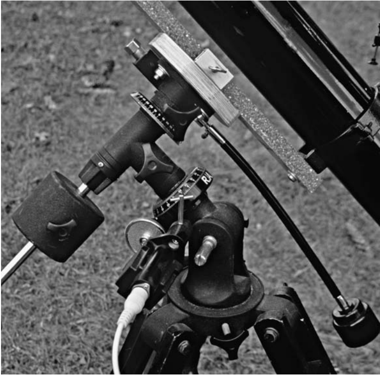
Figure 3.17 The CG-3 (or EQ-2) mount; this one is equipped with a single-axis drive. Note the slow-motion control cable angling downward to the right.
