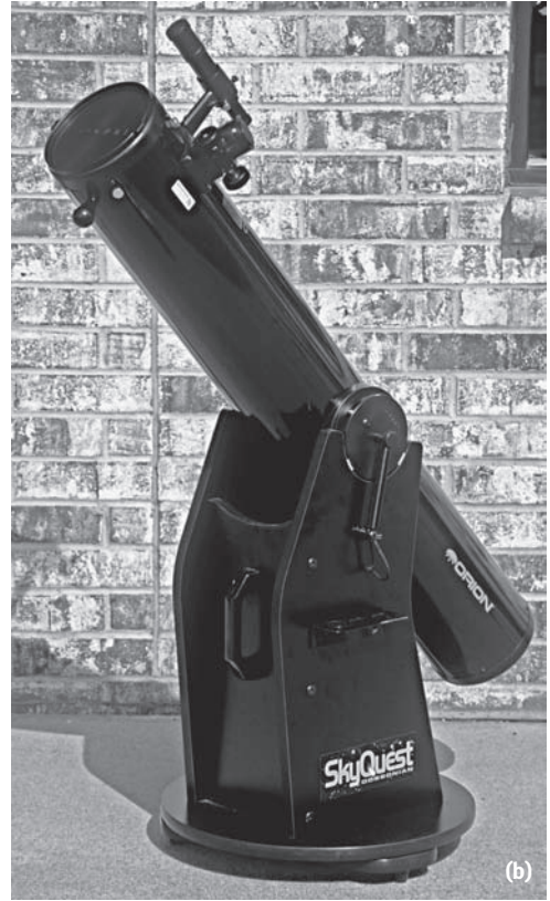
Figure 3.14 Alt-az mounts. (a) When you adjust the tension of the lever on top of the tripod, and the handle coming out from it, then you can easily turn the scope on this mount by hand, and have it stay where you put it. (b) A 6-inch (150-mm) reflector with a Dobsonian mount. You can easily adjust the aim of this scope by pushing and pulling on the round knob on the bottom of the front end.
