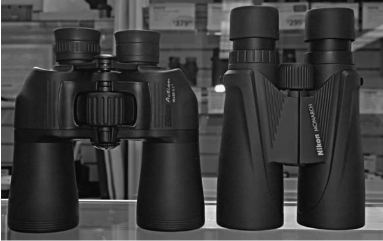
Figure 2.2 These two pairs of binoculars are comparable in size (10 × 50) and quality, but the pair on the right, with roof prisms, is priced three times higher than the pair on the left, which uses porro prisms.
