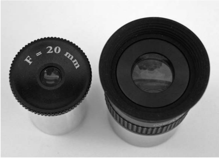
Figure 3.23 It is not just focal length that is responsible for short eye relief. The cheap, 0.965-inch eyepiece of unknown design on the left has a focal length of 20mm, but it has much less eye relief, and a much smaller eye lens, than the 1.25-inch, 15-mm focal length Plossl eyepiece on the right.
