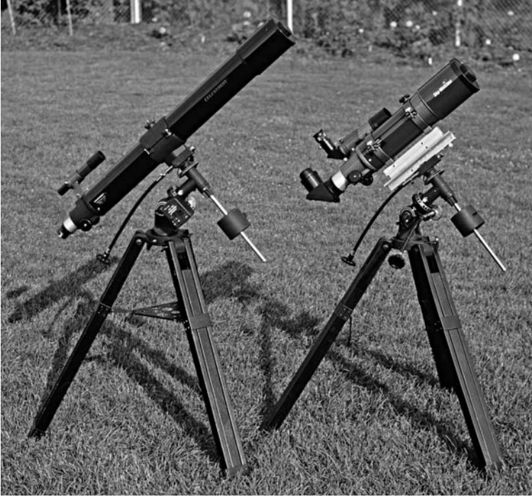
Figure 3.6 Two telescopes with different apertures, focal lengths, and focal ratios. The scope on the left, with an 80-mm aperture and 910-mm focal length (giving a focal ratio of about 11.4, when you divide the focal length by the aperture), is a good choice for a small, all-in-one scope for a beginner. It should be able to span a useful range of magnifications somewhere between 30 \times and 160 \times . The scope on the right, with an aperture of 100 mm, and a focal length of 500 mm (for a focal ratio of f/5 ) might seem like it could be used at higher magnification because of its larger aperture. But at f/5 , and with such a short focal length, it is much better suited for wide views, and can give stunning images at powers as low as 16 \times .
