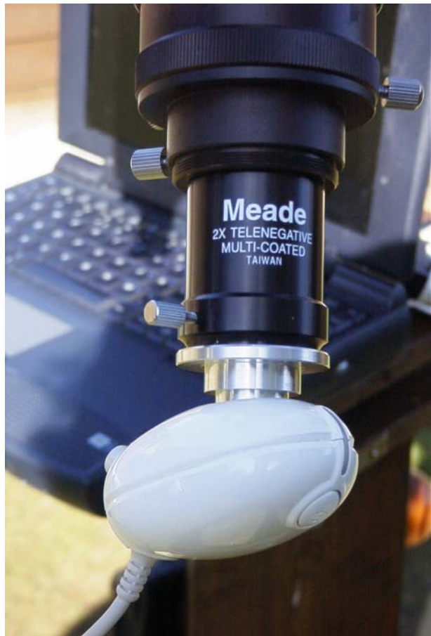
A Philips PCVC740 webcam set up with a Barlow lens at prime focus for lunar and planetary imaging. Peter Grego.
