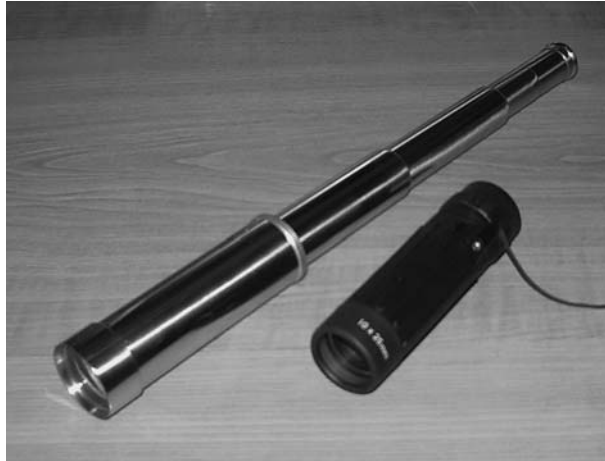
Two handy little telescopes – a brass drawtube 30 mm refractor with a 10–30 variable magnification, compared with a 10× 25 monocular. Peter Grego.
