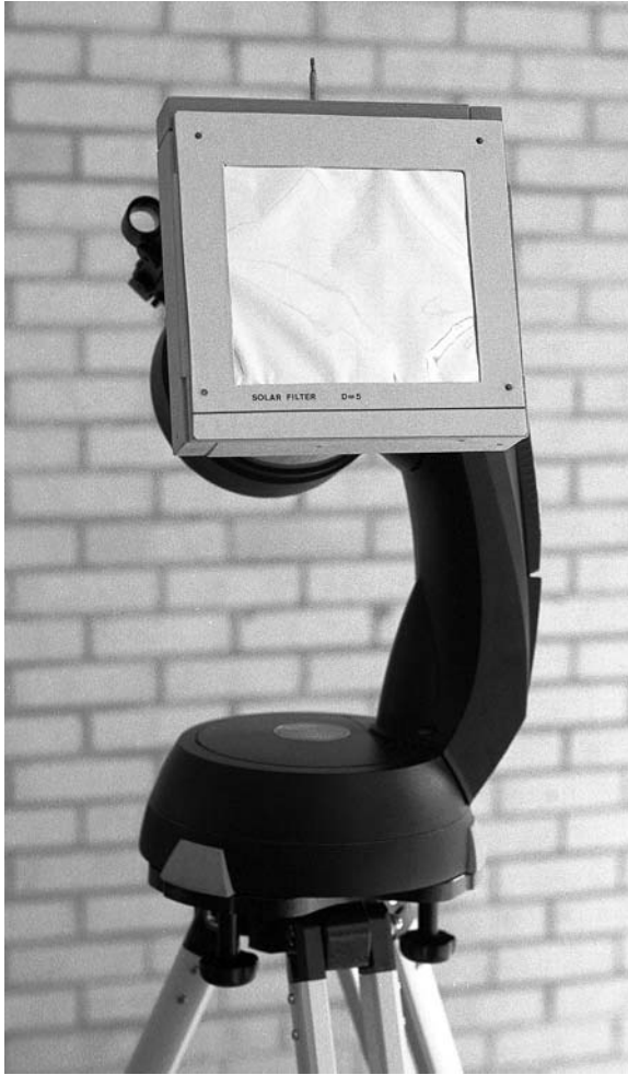
Figure 3.8. Mylar sun filter mounted in an improvised wooden cell.
