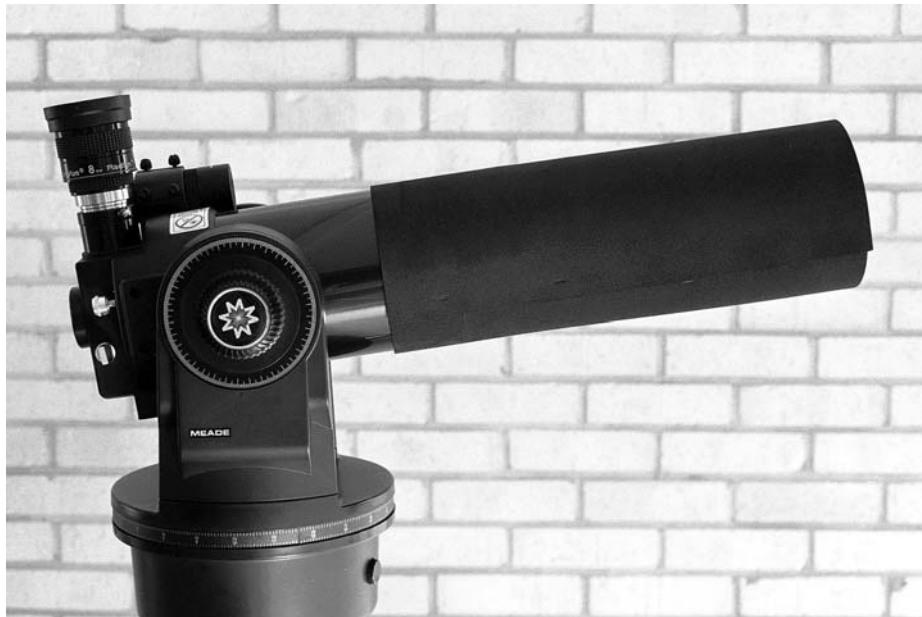
Figure 2.8. The dew cap of Cyrano de Bergerac, or perhaps Pinocchio. Half this length would be sufficient. This is plastic craft foam, but black paper would work almost as well.
