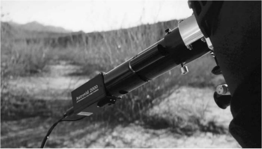
Figure 2.9. The Collins I 3 with the new video adapter, attached to my Astrovid 2000 CCD video camera and JMI 18 inch telescope at desert location.
