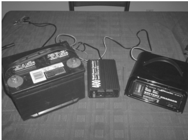
Figure 2.10. 12-volt, 480-amp battery, 400-watt inverter, and battery charger. Image by author.
