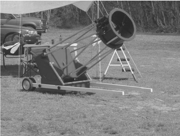
Figure 2.11. A large ATM-built Dobsonian at the Delmarva Stargazers star gaze star party. Image courtesy Delmarva Stargazers Yahoo Group.
