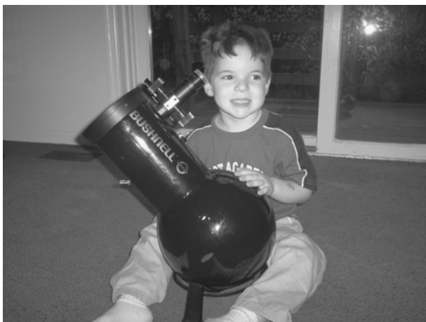
Figure 2.2. A short-focus Newtonian reflector. Image by author.
