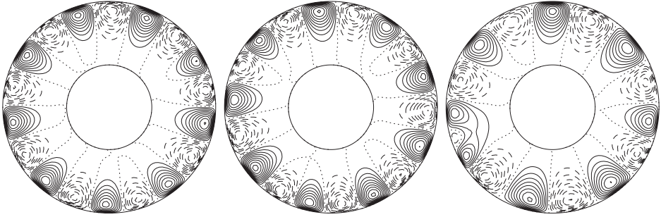
Figure 3.32 - Streamlines r \partial u_p / \partial \phi = \text{const.} in the equatorial plane for the case \text{Pr} = 0.025 , \tau = 10^5 with \text{Ra} = 3.2 \times 10^5 , 3.4 \times 10^5 , 4 \times 10^5 (from left to right).
