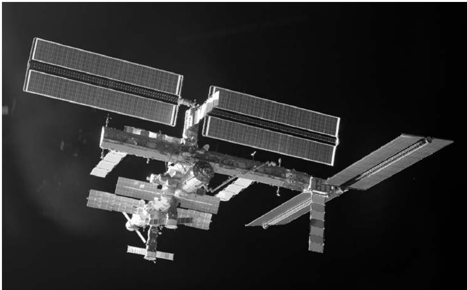
Figure 76. STS-115: construction has resumed. The station displays the new P-3/P-4 Solar Array Wings and ammonia radiator at right. Meanwhile, the Solar Array Wings and ammonia radiator are still deployed on the P-6 Integrated Truss Structure, mounted on the Z-1 Truss.
