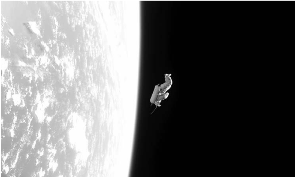
Figure 65. Expedition-12: A “past its sell-by date” Orlan pressure suit fitted with a radio transmitter was jettisoned to become a satellite in its own right. The experiment was named “RadioScaf”, but in their wisdom the media called it “Suitsat”.
