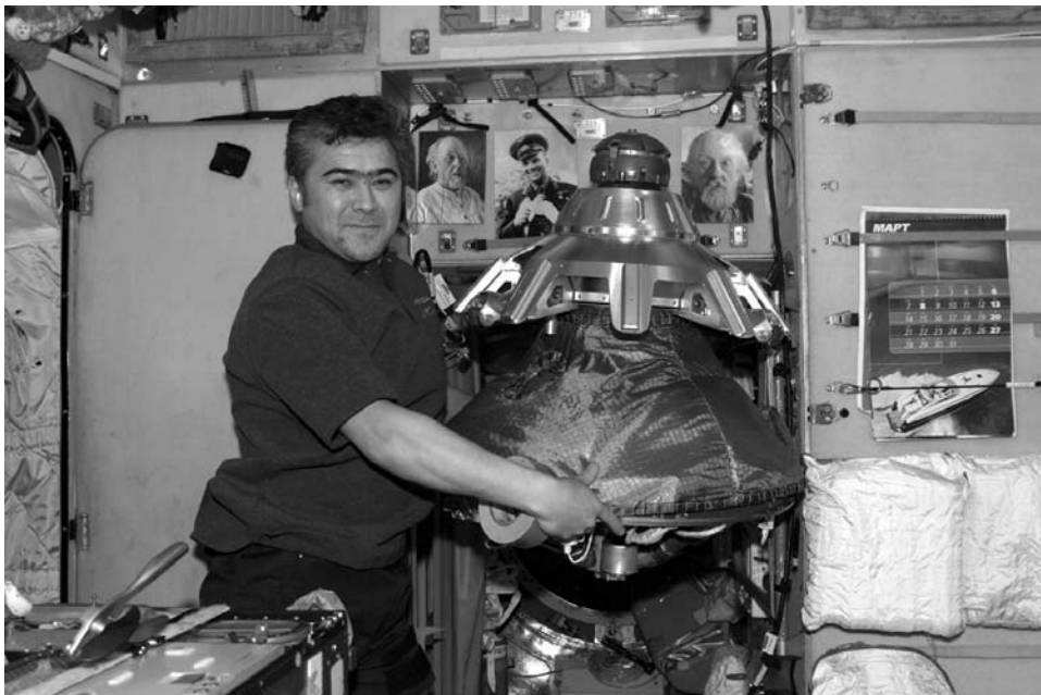
Figure 51. Expedition-10: Salizhan Sharipov holds a docking probe removed from a Progress cargo vehicle. It would be stored in Zarya until the Shuttle resumed flying, at which time it would be returned to Earth for refurbishment and re-use. The doorway on the left-hand edge of the frame gives access to one of Zvezda's two sleeping quarters. Note the picture of Russian spaceflight pioneers Konstantin Tsiolkovsky and Yuri Gagarin on the wall behind him.
