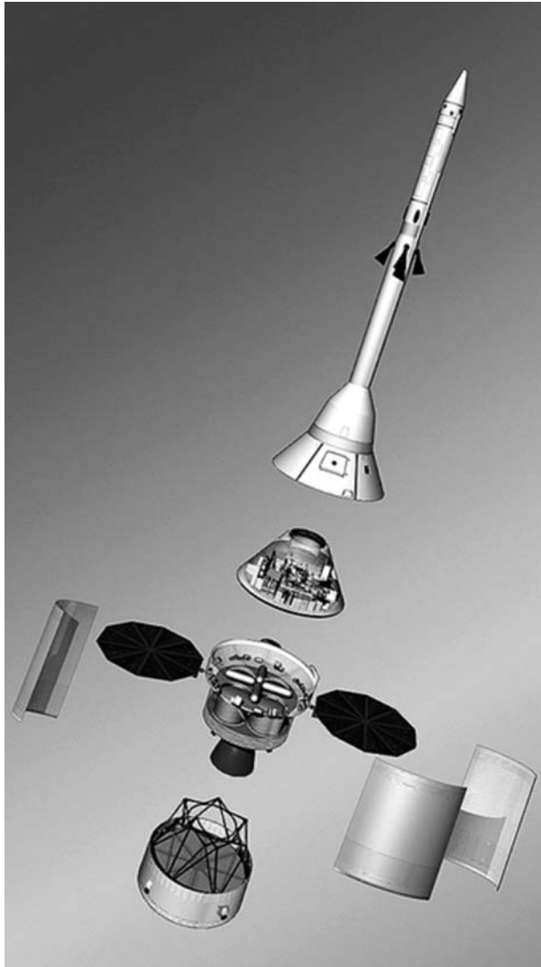
Figure 111. Constellation (early concept): the component parts of the new Orion spacecraft are from top to bottom: Launch Abort System with Boost Protection Cover, Crew Compartment, Service Module with circular Solar Array Wings, and launch vehicle adapter.
