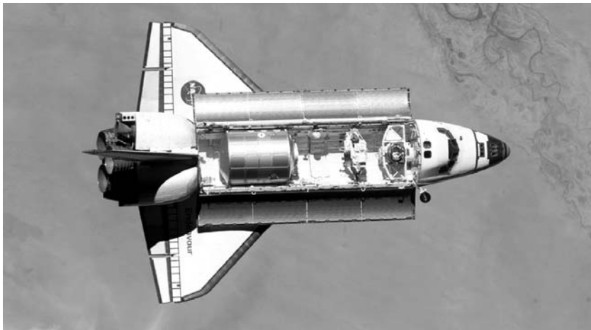
Figure 19. STS-111: Endeavour delivers the Multi-Purpose Logistics Module Leonardo to the International Space Station.
