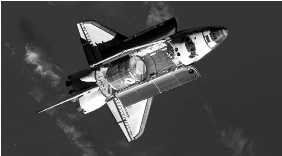
Figure 103. STS-120 approaches ISS with Node 2, Harmony, in the payload bay.
