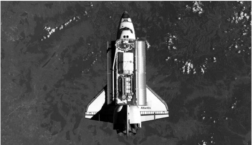
Figure 74. STS-115 approaches the ISS carrying the P-3/P-4 Integrated Truss Structure.
