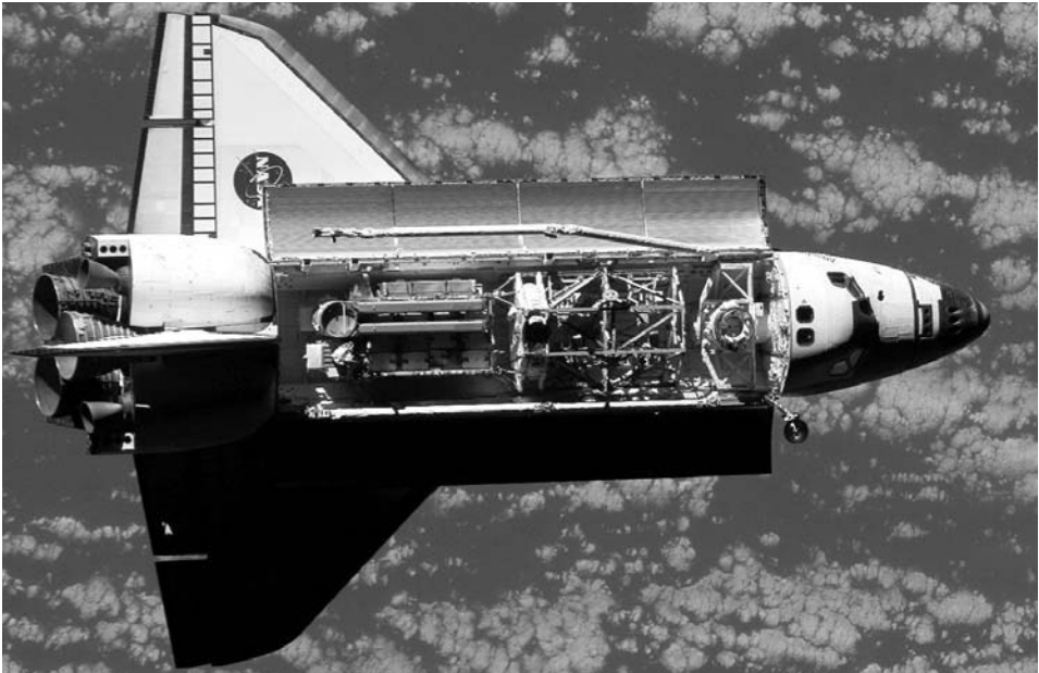
Figure 89. STS-117 delivers the S-3/S-4 Integrated Truss Structure to ISS.
