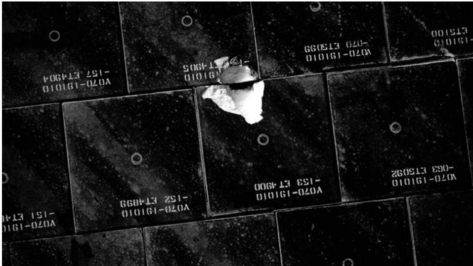
Figure 99. STS-118: the decision was made not to repair this tile damage on Endeavour’s underside. The damage to the orbiter’s heat protection system had no effect on re-entry, and Endeavour was recovered successfully.
