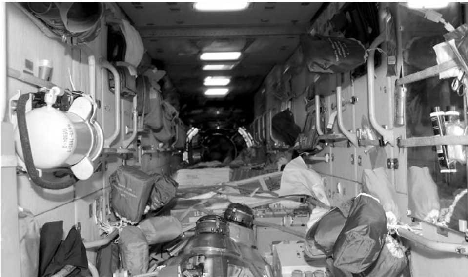
Figure 53. Expedition-10: note the two Progress docking probes in the foreground of the Zarya image. Only the Shuttle could return bulky items such as these to Earth. Zvezda was equally cramped by this time.
