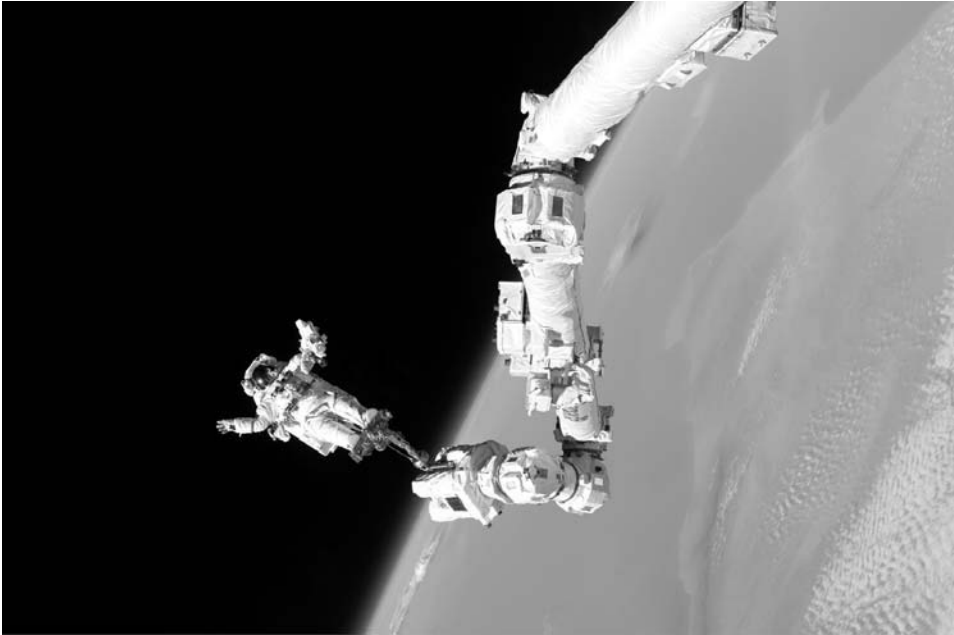
Figure 61. STS-114: Robinson rides the SSRMS during the flight's second extravehicular activity.
