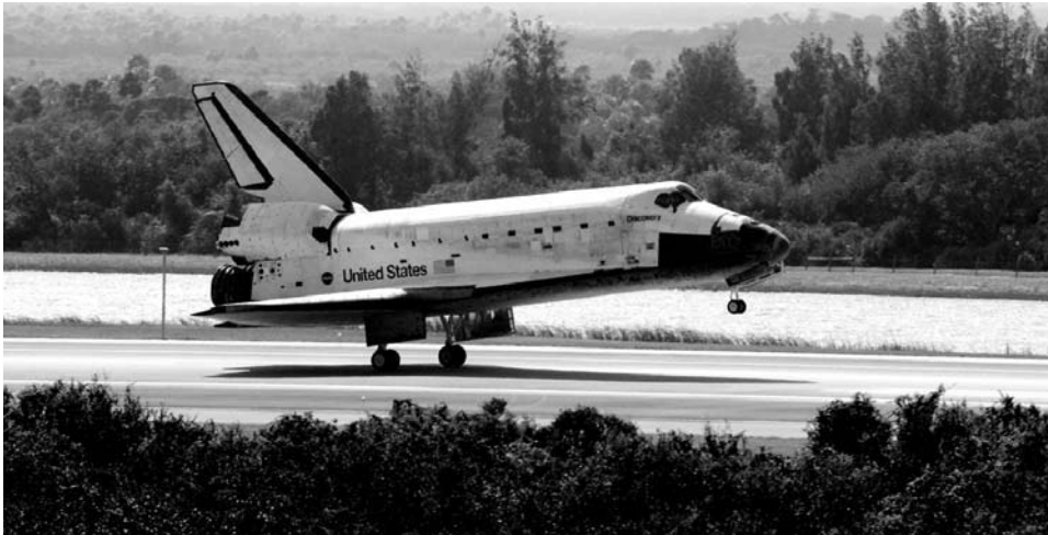
Figure 2. After re-entry through Earth's atmosphere the Shuttle orbiter approaches the landing strip along a trajectory that is far steeper and faster than a commercial airliner.
