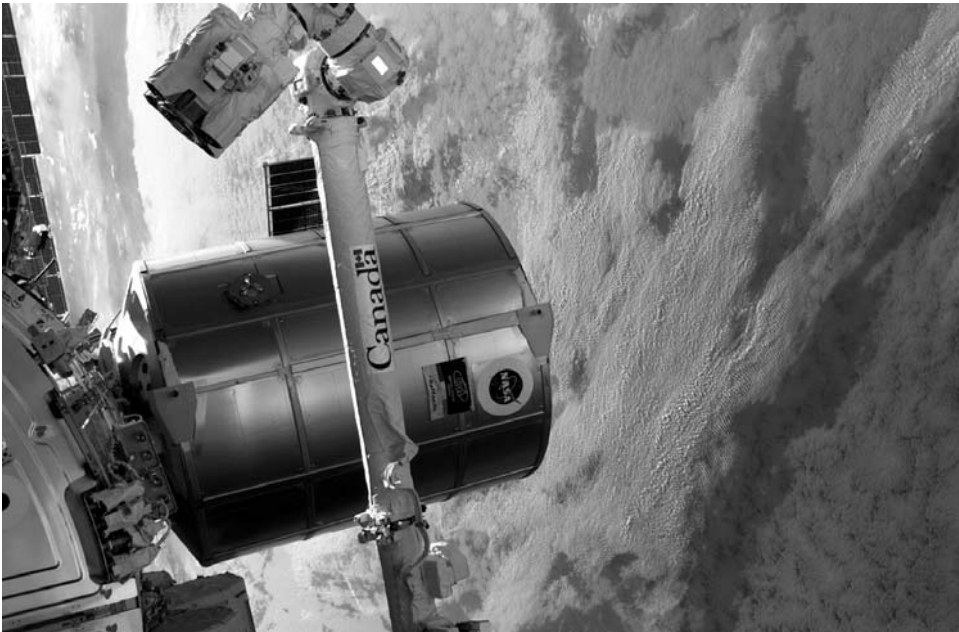
Figure 8. Multi-Purpose Logistics Modules were removed from the Shuttle's payload bay and docked to Unity before being unloaded via an internal hatch. The empty module was then filled with items no longer required on the station and returned to the Shuttle's payload bay for return to Earth.
