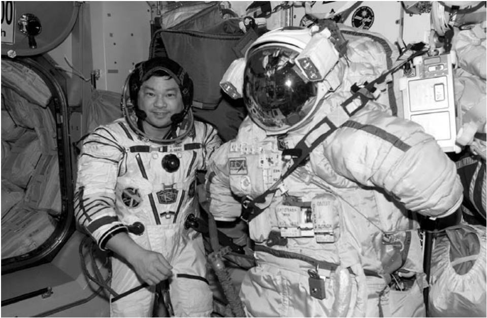
Figure 48. Expedition-10: Leroy Chiao wears his Sokol launch and re-entry suit while posing alongside a Russian Orlan extravehicular activity suit.
