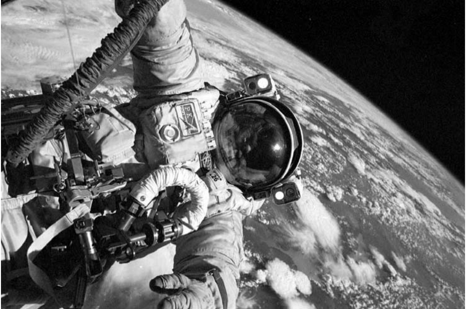
Figure 46. Expedition-9: Gennady Padalka wears a Russian Orlan suit during the Expedition-9 crew's third two-man extravehicular activity.
