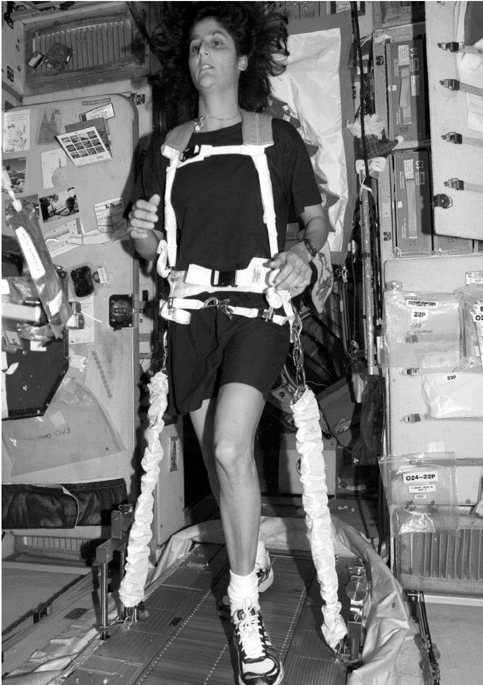
Figure 84. Expedition-14: Sunita Williams runs on the treadmill in Zvezda. The elastic harness keeps her in place in the microgravity environment.
