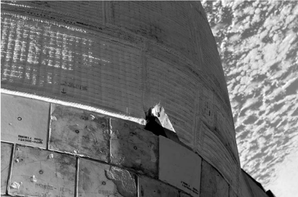
Figure 93. STS-117: image shows the protruding corner of a thermal blanket on the orbiter's OAMS pod.
