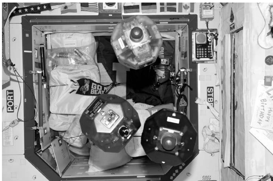
Figure 83. Expedition-15: three SPHERES micro-satellites float in Zvezda during testing.
