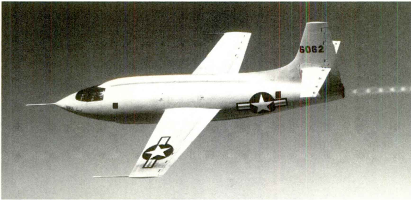
11. The Bell Aircraft X-1 in flight in 1947. The shock-wave pattern in the exhaust plume is visible. The X-1 series aircraft were air-launched from modified Boeing B-29 Superfortress bombers. Air force pilot Chuck Yeager broke the sound barrier for the first time while flying an X-1. (NASA photo)
