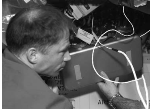
Rick Searfoss and Scott Altman (out of frame) repair the Regenerative Carbon Dioxide Removal System (RCRS).
