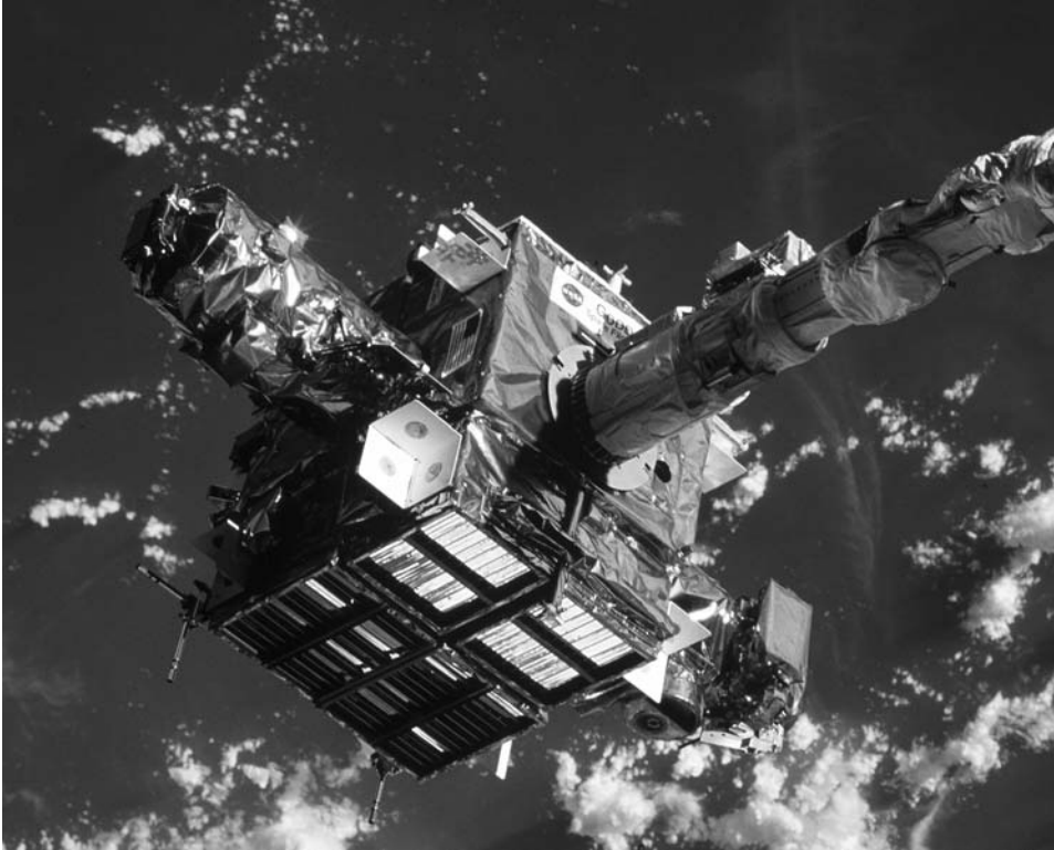
Firmly held by the RMS, the Spartan-201 satellite awaits deployment.
