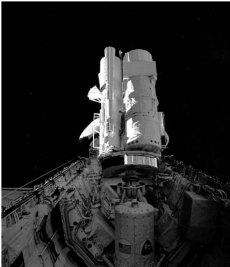
The ASTRO-1 observatory at work during STS-35. Note the cylindrical igloo at the front of the first Spacelab pallet.
