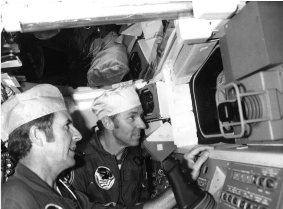
Dick Truly (left) and Joe Engle in the Shuttle simulator’s aft flight deck practise operating the RMS.
