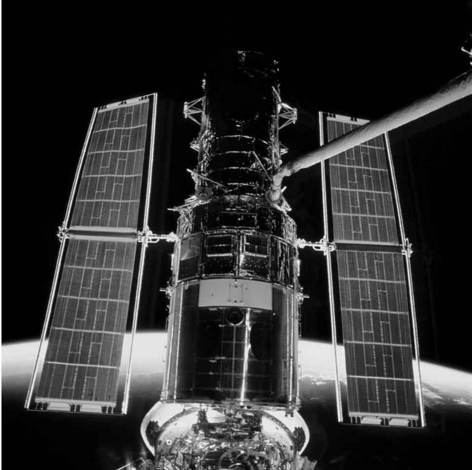
Deftly manipulated by Nancy Currie, Columbia's RMS mechanical arm has Hubble firmly in its grasp.
