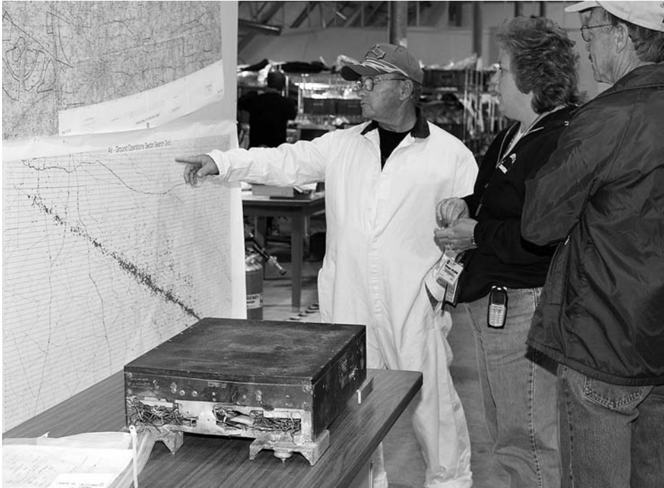
The recovered Orbiter Experiments (OEX) recorder: battered, but in one piece. It was to provide key evidence for what had happened to Columbia in her final minutes.
