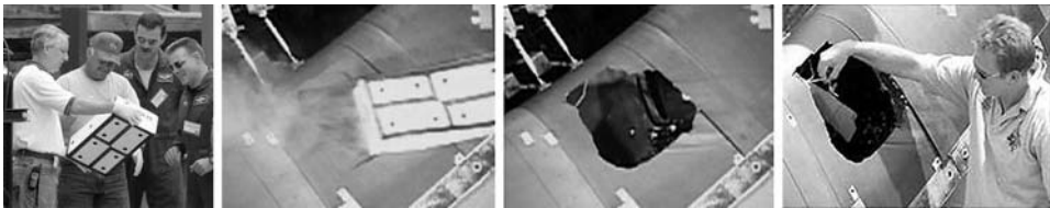
Series of images of a damaged RCC panel following a foam-strike test at the Southwest Research Institute (SWRI) on 7 July 2003.
