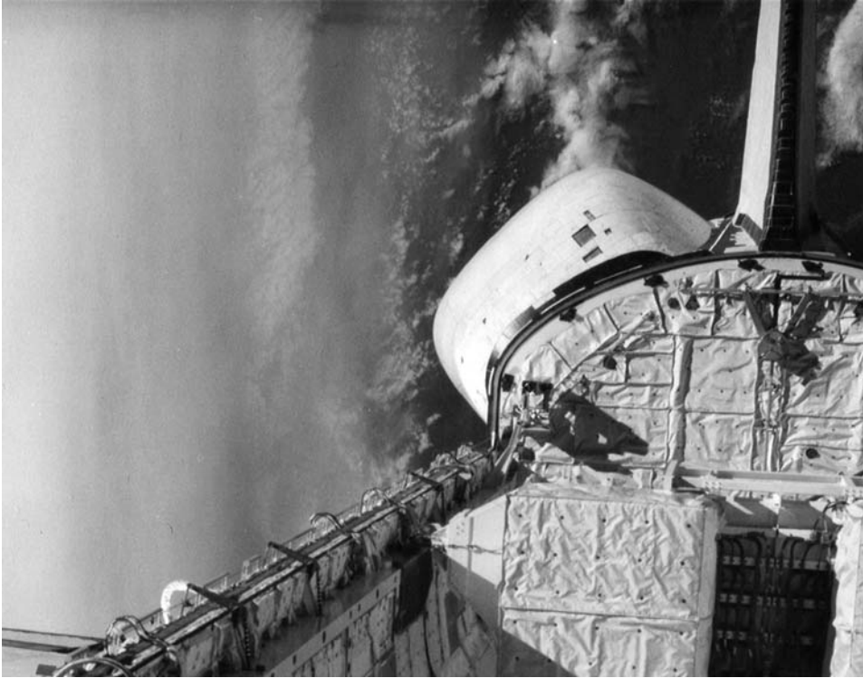
View of Columbia's payload bay, revealing missing tiles from her OMS pods. Note the two boxes, which form part of the DFI package.
