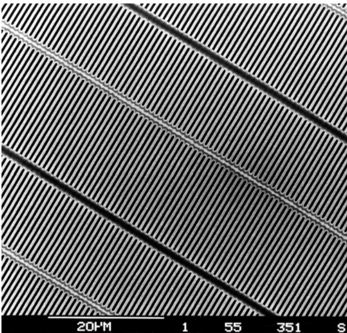
Fig. 8.3 Electron microscope image of a freestanding transmission grating with 1000 lines per millimeter. The grating bars are held by support grid having a pitch of 25 μm (courtesy DR. JOHANNES HEIDENHAIN GmbH)
