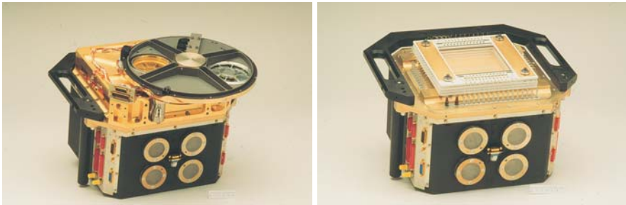
Fig. 4.5 The position sensitive proportional counter of the ROSAT telescope with closed and open detector housing [18]
