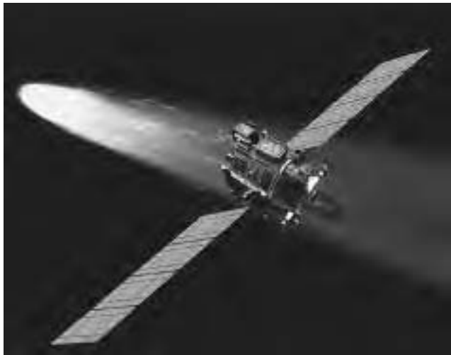
This artist's rendering depicts NASA's New Millennium Deep Space 1 (DS1) spacecraft approaching Comet 19P/Borrelly in September 2001. With its primary mission to serve as a space technology demonstrator—especially the flight testing of an advanced xenon electric propulsion system and 11 other advanced aerospace technologies—successfully completed by September 1999, Deep Space 1 headed for a risky, exciting rendezvous with Comet Borrelly. On September 22, 2001, the Deep Space 1 spacecraft entered the coma of Comet Borrelly and successfully made its closest approach, a distance of about 2,200 km, to the nucleus at about 22:30 UT (6:30 P.M. EDT). At the time of the encounter, DS1 was traveling at 16.5 km/s relative to the comet's nucleus. (Courtesy of NASA/JPL)
