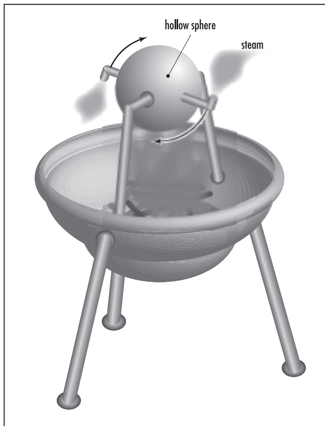
In about 60 C.E. the Greek engineer and mathematician Hero of Alexandria created the aeoliphile (shown here), a toylike device that demonstrates the action-reaction principle, which is the basis of operation of all rocket engines.
