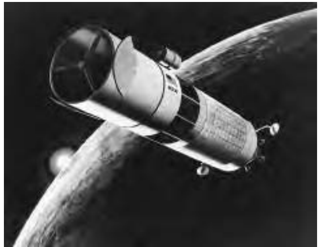
Artist's rendering of a space-based, high-energy laser system (ca. 2020) that would intercept enemy ballistic missiles in the boost phase, before they can deploy their warheads and decoys (Courtesy of the U.S. Department of Defense)
