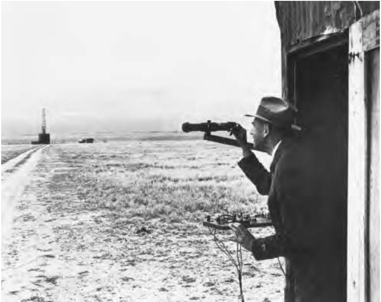
Dr. Robert H. Goddard observes a rocket test from his launch control shack site in the New Mexican desert near Roswell. While standing by the firing control panel, Goddard could fire, release, or stop testing his rocket if conditions became unsatisfactory. The firing, releasing, and stopping keys are shown on the control panel. In this 1930s-era photograph Goddard is using a small telescope to view the launch of one of his pioneering liquid-propellant rockets, which is located in the launch tower in the distance. (Courtesy of NASA)
