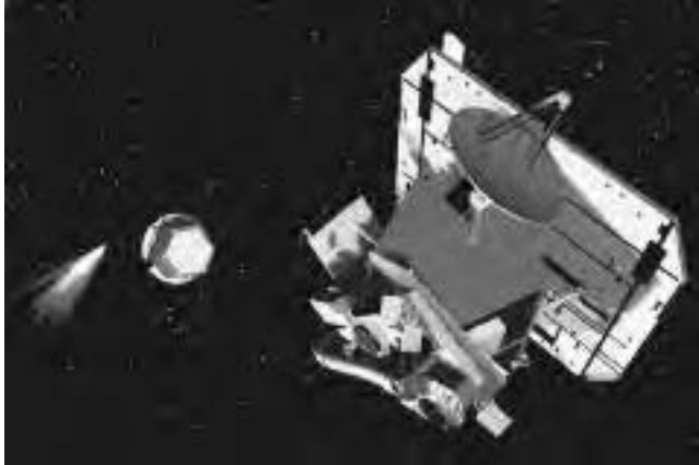
This is an artist's rendition of the Deep Impact flyby spacecraft releasing the impactor 24 hours before the impact event. Pictured from left to right are Comet Tempel 1, the impactor, and the flyby spacecraft. The impactor is a 370-kilogram mass with an onboard guidance system. The flyby spacecraft includes a solar panel (right), a high-gain antenna (top), a debris shield (left, background), and science instruments for high- and medium-resolution imaging, infrared spectroscopy, and optical navigation (box and cylinder, lower left). The flyby spacecraft is about 3.2 meters long, 1.7 meters wide, and 2.3 meter high. The launch payload has a mass of 1,020 kilograms. (Courtesy of NASA/JPL/UMD)
