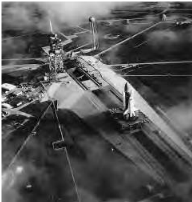
A panoramic early-morning view of Complex 39 (Pad A) at the Kennedy Space Center in Florida as an assembled space shuttle vehicle nears the completion of its nearly six-kilometer-long slow rollout journey from the Vehicle Assembly Building (VAB) to the launch pad. Shown here is the Challenger on November 30, 1982. (Courtesy of NASA)
