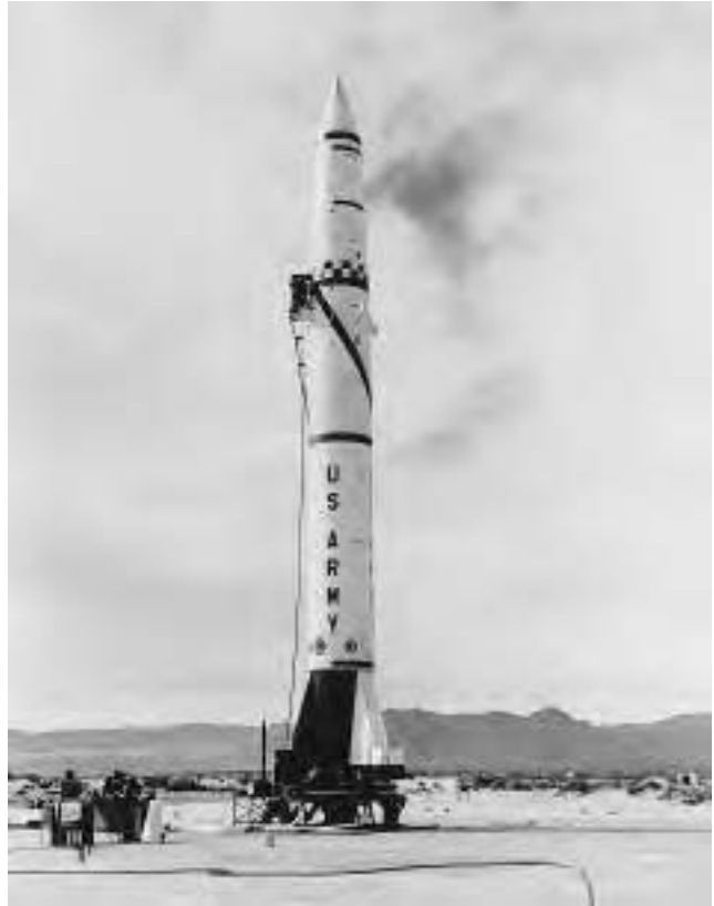
U.S. Army personnel prepare to launch a Redstone intermediate-range ballistic missile (IRBM) at the White Sands Missile Range in the early 1950s. A direct technical descendent of the German V-2 military rocket, the Redstone rocket also was pressed into service as a space launch vehicle, helping to successfully place the first American satellite, Explorer 1 , into orbit in 1958 and then propelling the Project Mercury astronauts Alan B. Shepard, Jr. and Virgil “Gus” I. Grissom on the first two successful American manned space missions (both suborbital) in 1961. (Courtesy of the U.S. Army)
