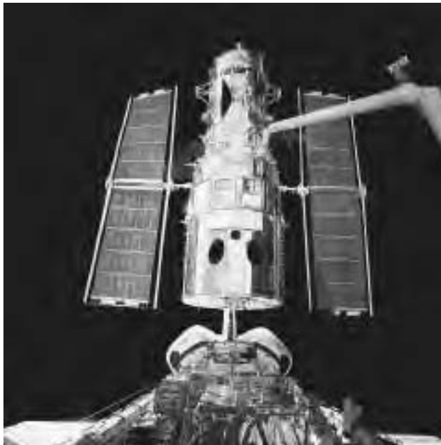
NASA's Hubble Space Telescope (HST) being unberthed and carefully lifted up out of the payload bay of the space shuttle Discovery and then placed into the sunlight by the shuttle's robot arm in February 1997. This event took place during the STS-82 mission, which NASA also calls the second HST servicing mission (HTS SM-02). (Courtesy of NASA/JSC)
