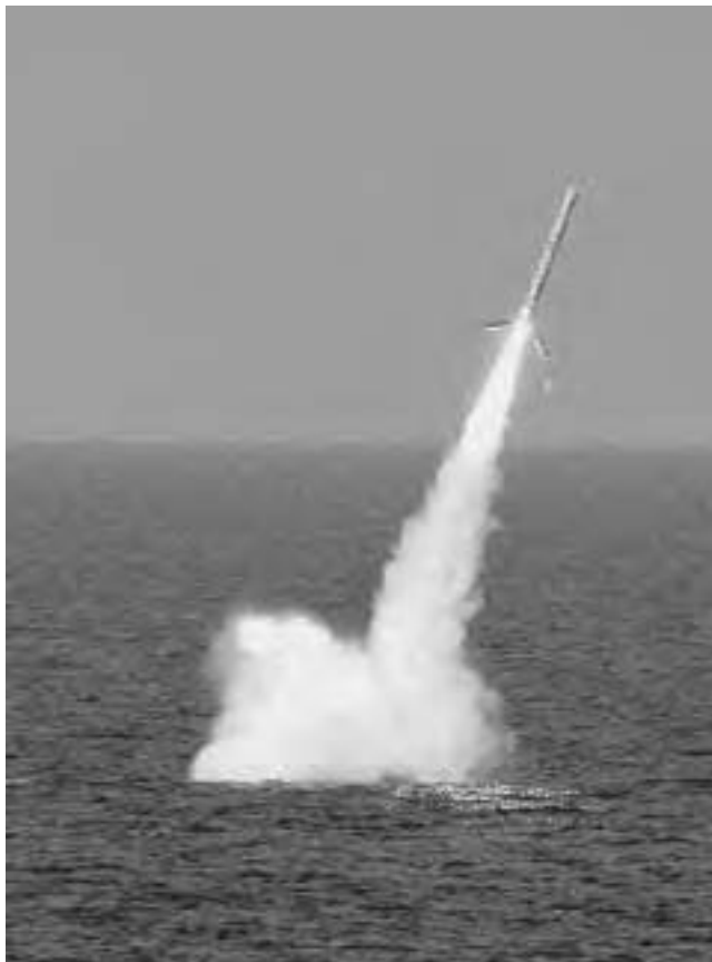
During a submerged exercise off the coast of the Bahamas in January 2003, the nuclear-powered ballistic missile submarine USS Florida launched a Tomahawk cruise missile to test the capabilities of the U.S. Navy's guided missile submarines. The USS Florida is one of four Ohio-class ballistic missile submarines (designated SSBN) being converted to guided missile submarines (designated SSGN). The SSGNs will have a capability to support and launch up to 154 Tomahawk guided missiles. (Courtesy of the U.S. Navy)
