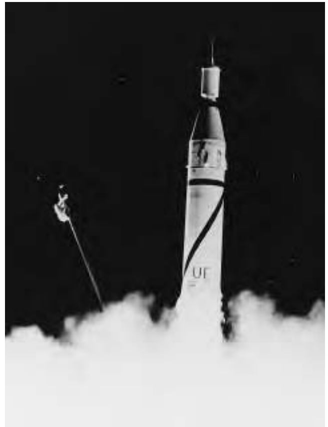
Late in the evening on January 31, 1958 (local time), this four-stage configuration of the Jupiter C rocket blasted off from Cape Canaveral Air Force Station and successfully placed the Explorer 1 spacecraft, the first United States satellite, into orbit around Earth. (Courtesy of NASA)
