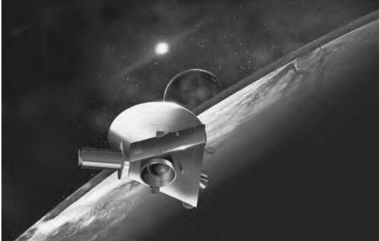
This is an artist's rendering of NASA's New Horizons spacecraft during its planned encounter with the tiny planet Pluto (foreground) and its relatively large moon, Charon, possibly as early as July 2016. A long-lived, plutonium-238 fueled, radioisotope thermoelectric generator (RTG) subsystem (cylinder on lower-left portion of the spacecraft) provides electric power as it flies past these distant icy worlds billions of kilometers from the Sun. As depicted here, one of the spacecraft's most prominent design features is a 2.1-meter-diameter dish antenna through which it communicates with scientists on Earth from as far as 7.5 billion kilometers away. Following its encounter with the Pluto-Charon planetary system, the spacecraft is hoped to encounter one or several icy planetoid targets of exploration in the Kuiper Belt. (Artwork courtesy of NASA/JPL)
