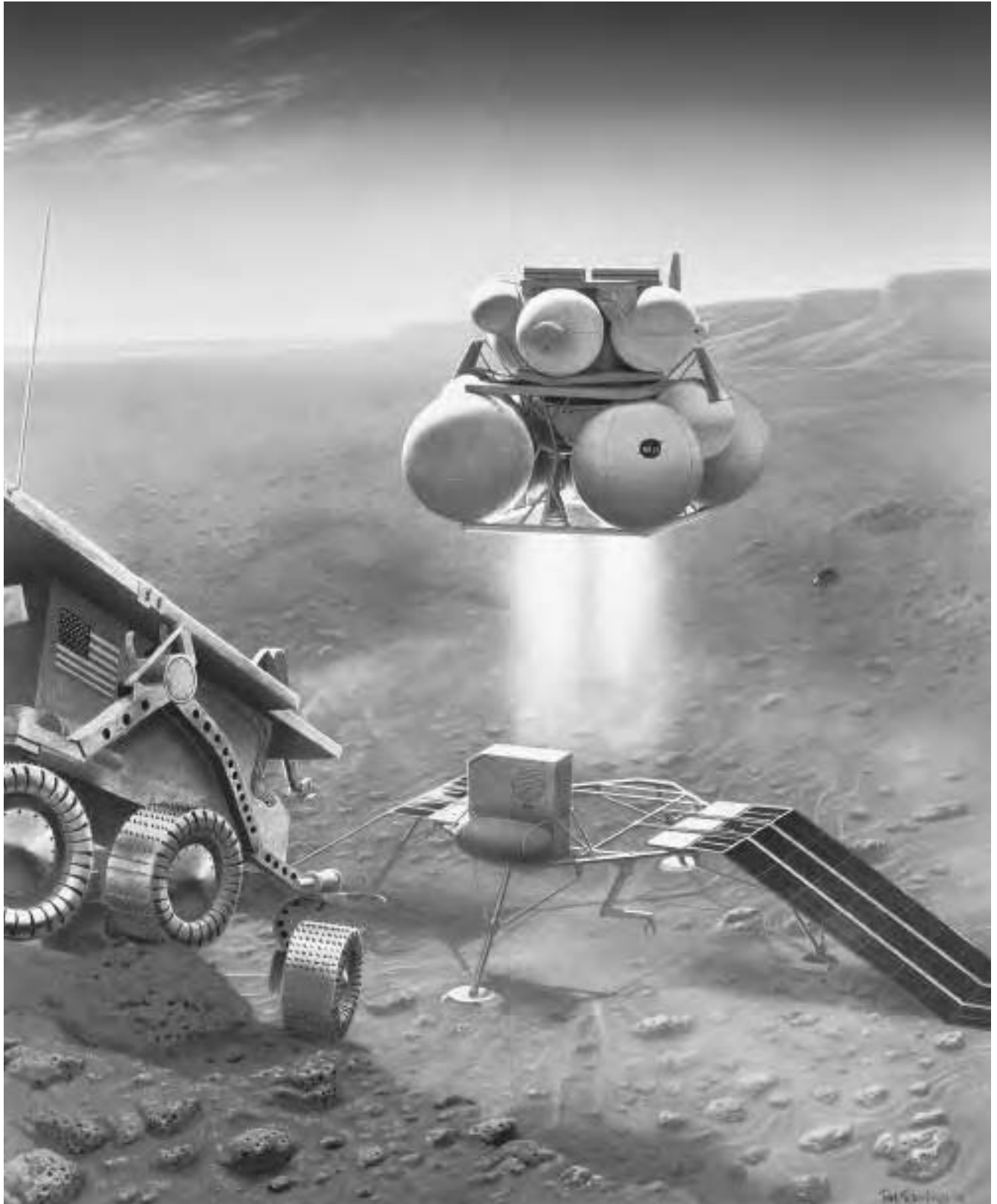
Artist's rendering of a Mars Sample Return Mission (MSRM). The sample return spacecraft is shown departing the surface of the Red Planet after soil and rock samples previously gathered by robot rovers have been stored on board in a specially sealed capsule. To support planetary protection protocols, once in a rendezvous orbit around Mars the sample return spacecraft would use a mechanical device to transfer the sealed capsule of Martian soil samples to an orbiting Earth-return spacecraft ("mother ship") that would then take the samples to Earth. (Artist's rendering courtesy of NASA/JPL; artist, Pat Rawlings)
