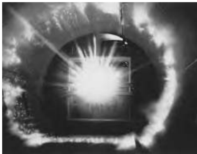
This photograph shows the “energy flash” when a hypervelocity particle traveling at speeds up to 7.5 km/s impacts a solid surface. Starting in 1963, NASA scientists at the Ames Research Center (ARC) performed this and similar tests to simulate what would happen when a small piece of space debris hits a spacecraft in orbit around Earth. (Courtesy of NASA/ARC)
