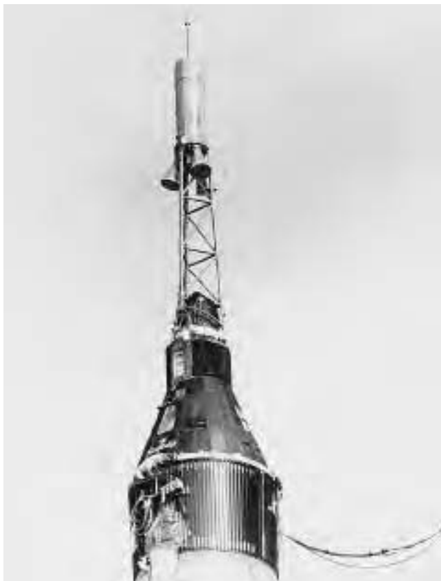
A close-up view of the escape tower attached to astronaut John Glenn's Friendship 7 space capsule as the two were mated to an Atlas rocket at Cape Canaveral in February 1962. Glenn became the first American to orbit Earth in a spacecraft as part of NASA's Mercury Project. ( Courtesy of NASA )
