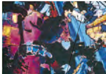
Cross-polarized light in the microscope gives colors Watery clearness shows no weathering
