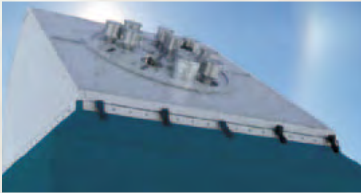
Solar array shields telescope from Sun's heat
