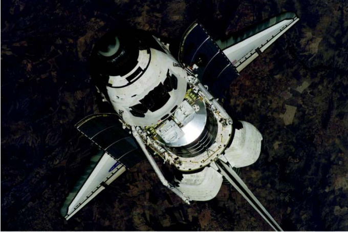
The Space Shuttle Discovery approaching the International Space Station for docking in July 2006. A module for the Space Station can be seen in the Shuttle's cargo bay.
