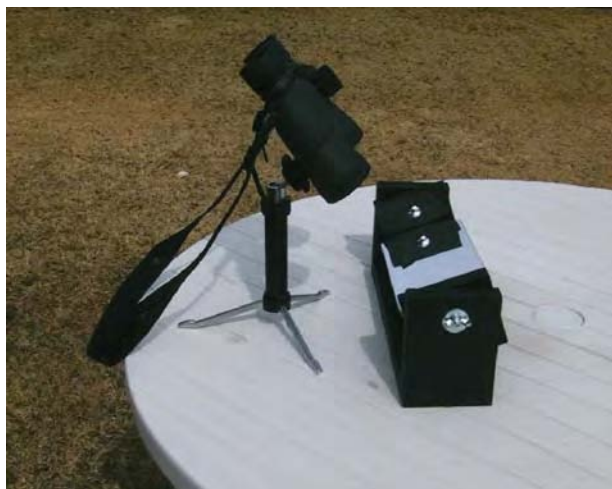
Figure 6.12. A homemade mirror mount (Photo: Florian Boyd).
