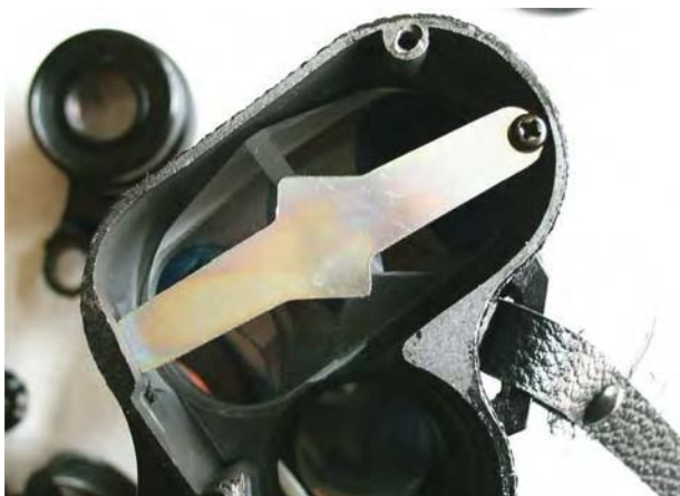
Figure 5.9. Clamped prism in Zeiss-type binoculars.
