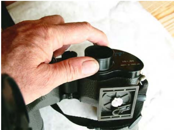
Figure 5.7. The eyepiece guide tubes are removed.
