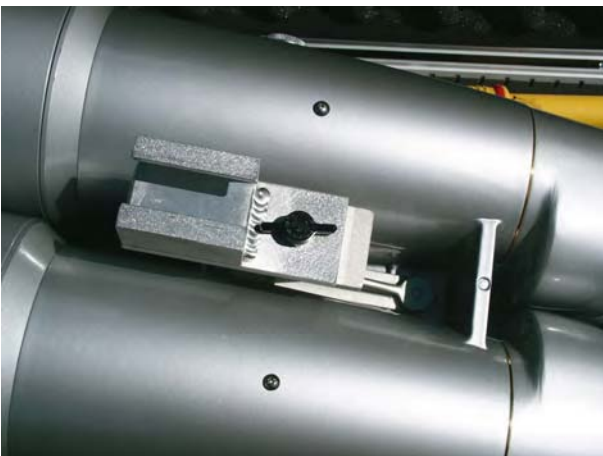
Figure 3.5. Bracket attached to mounting plate at the bottom of 20/37×100 binoculars.
