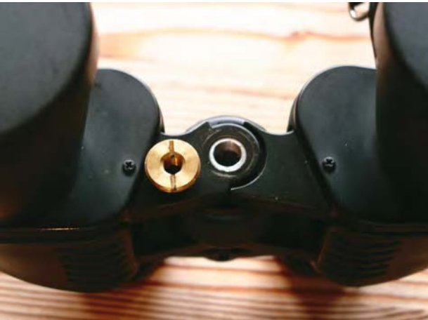
Figure 5.4. Tripod bush removed. This gives access to the screw that secures the focus shaft.
