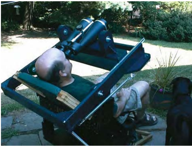
Figure 6.15. Homemade observing chair. Craig Simmons’s chair features a rotating base and spring counterweighting for the binoculars. Notice also how the altitude pivot axis coincides with the axis at the top of the observer’s spine. (Photo: Craig Simmons).
