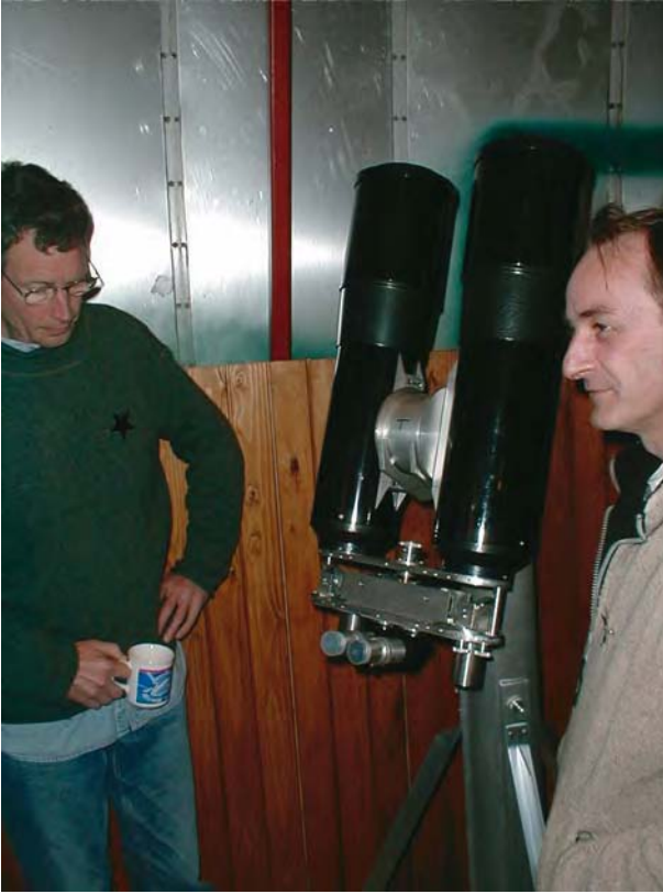
Figure 3.7. Binocular telescope by Peter Drew constructed from two 150mm (6 inch) Synta telescopes.
