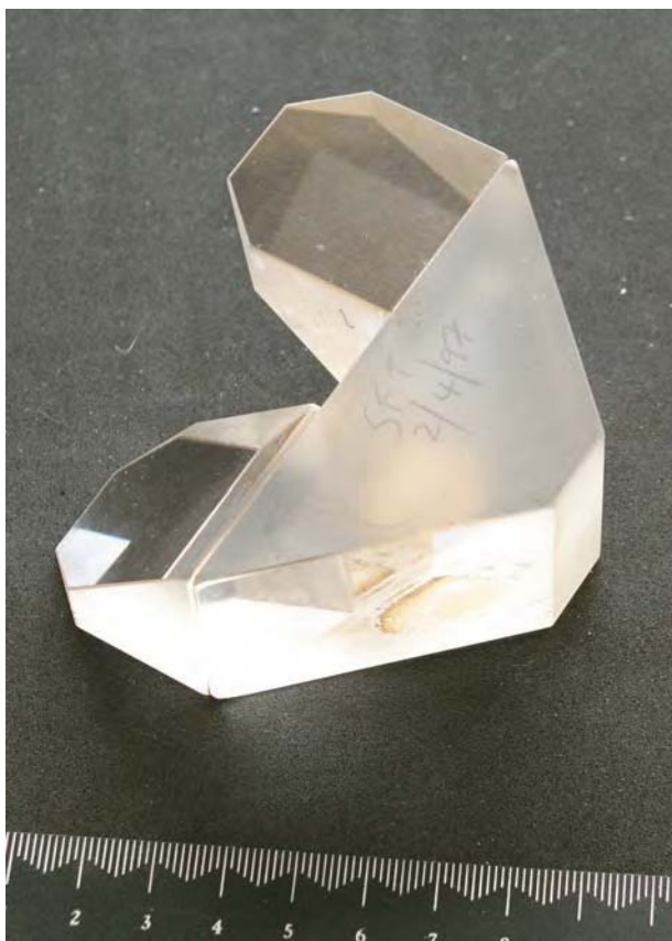
Figure 2.5. Abbé Erecting System, also known as a Porro Type-2 prism.
