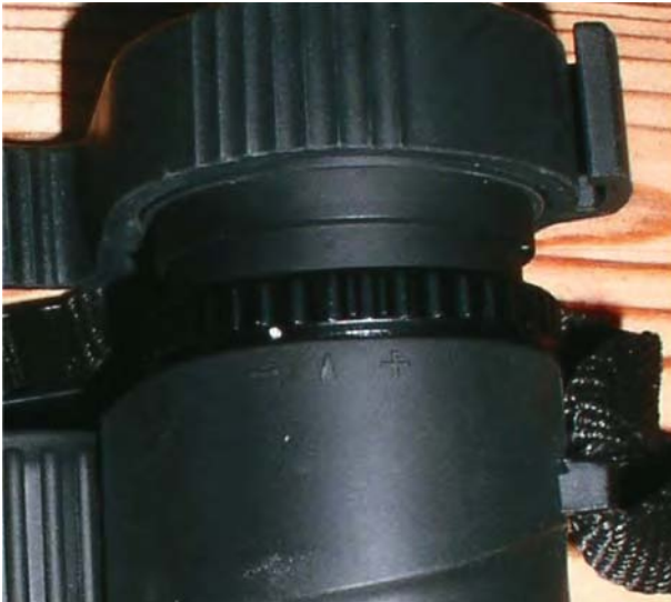
Figure 2.26. Right eyepiece diopter adjustment. a: Porro prism. b: Roof prism.
