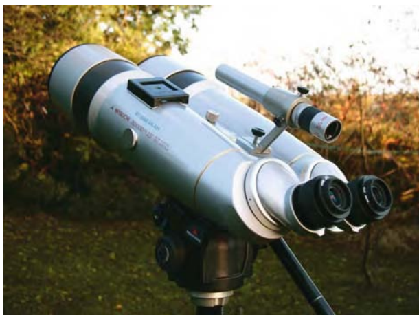
Figure 7.2. 3×12 finder scope with 55-mm eye relief.
