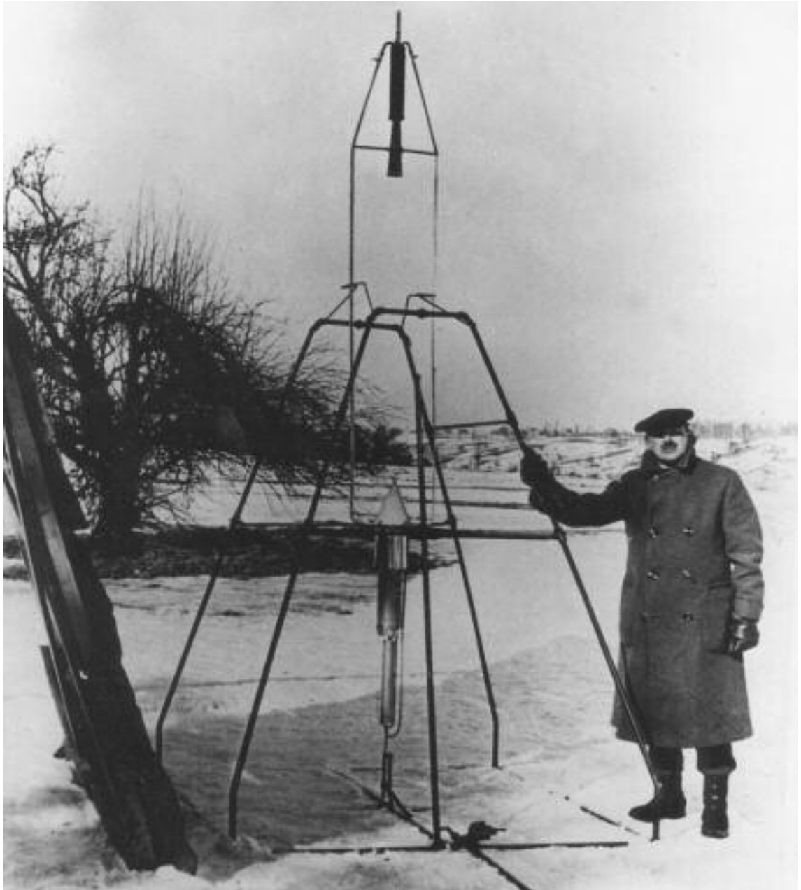
Robert H. Goddard and the world's first liquid propellant rocket in its launch frame. On March 16, 1926, Goddard successfully flight-tested this historic liquid oxygen-gasoline rocket in a field at Auburn, Massachusetts. From 1930 to 1941 he made substantial progress in the development of larger liquid-propellant rockets. With his pioneering experiments he developed and demonstrated the fundamental principles of modern rocket technology. Along with visionary theoreticians Konstantin Tsiolkovsky and Hermann Oberth, Goddard is regarded as one of the founding fathers of astronautics. (Courtesy of NASA)
