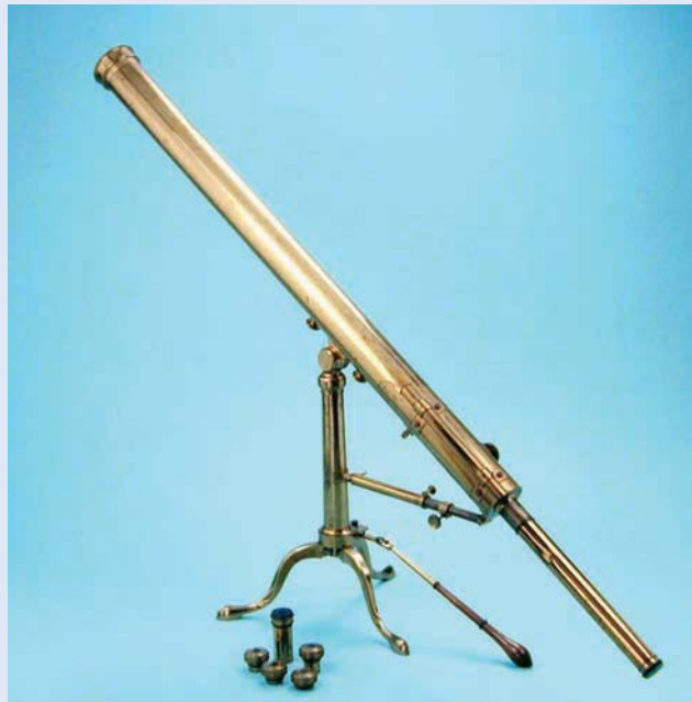
Dollond refractors, the first achromatic refractors produced in large numbers, arrived on the optical market in 1758. Messier used such a telescope with 90mm (3.5 inches) of aperture for many of his deep-sky observations.
