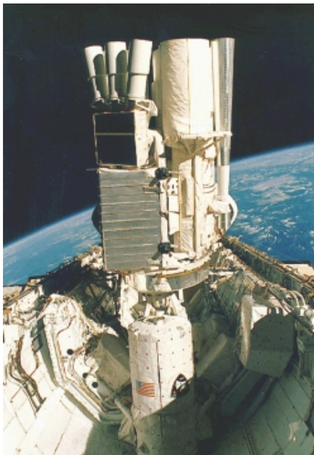
Figure A.2 Astro-1 instruments in the Space Shuttle Bay. UIT is the large cylinder blanketed with thermal insulation. Credit: STScI and NASA.
