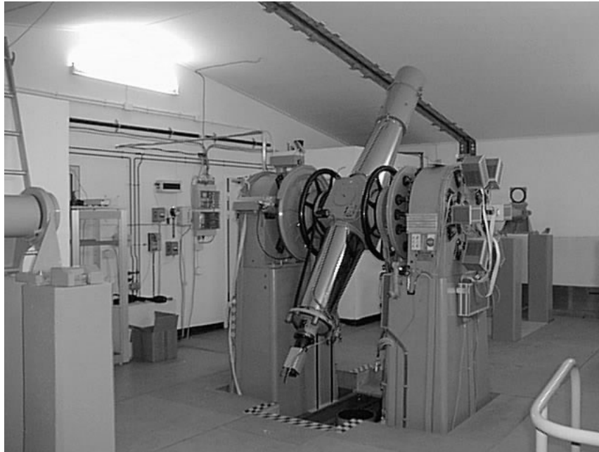
Figure 20.11. The Carlsberg Meridian Telescope with CCD detector system attached for the automatic monitoring of stellar transits. Both positions and brightnesses of over 100 000 stars are regularly recorded each night.
