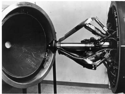
An engineering model of the probe and drogue docking mechanism.
