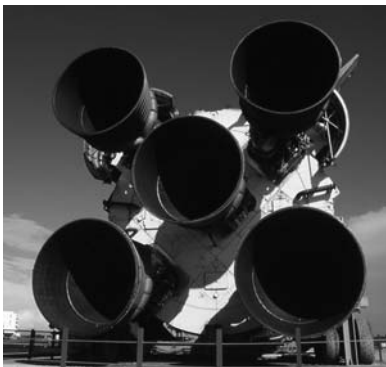
Five F-1 engines at the base of an S-IC first stage.
