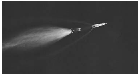
Apollo 11's S-IC stage falls away as the S-II takes over.
