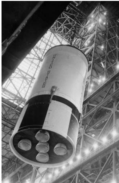
Apollo 10's S-II stage about to be stacked as part of the launch vehicle.
