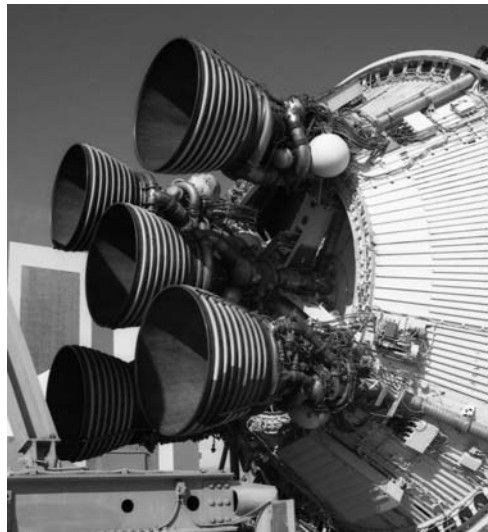
The five J-2 engines at the base of an S-II stage.
