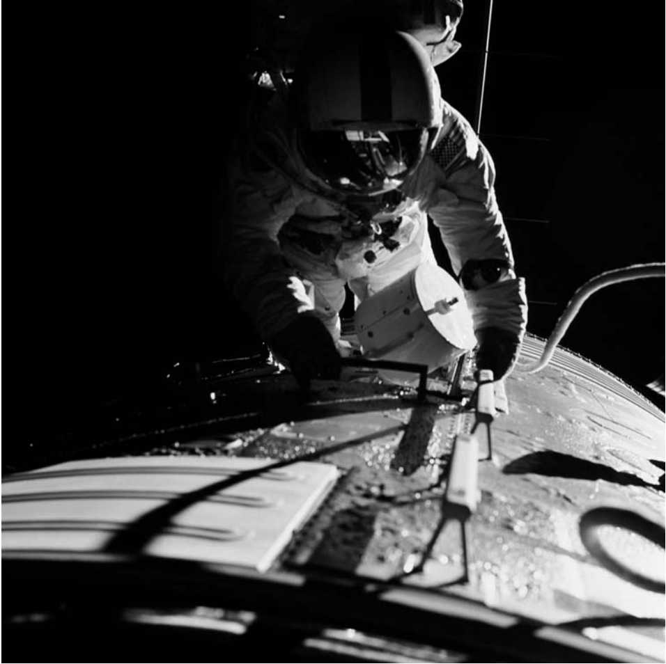
Ron Evans returning along the side of the Apollo 17 SM carrying the cassette from the mapping camera.
