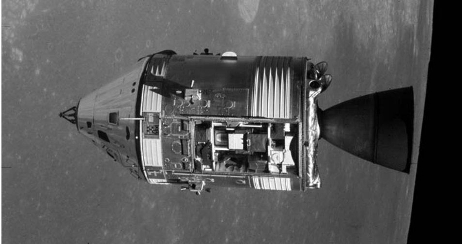
The Apollo 15 CSM Endeavour showing its SIM bay.
