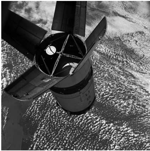
Apollo 7's S-IVB had no LM but included a target for docking practise.
