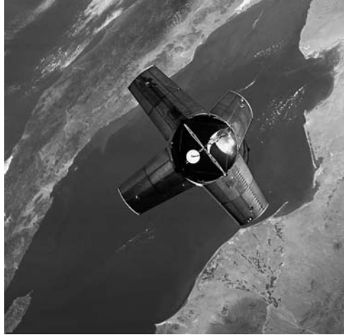
Apollo 7's S-IVB and its deployed shroud petals.
