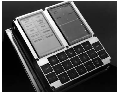
A display and keyboard (DSKY), a crew’s interface with the computer.
