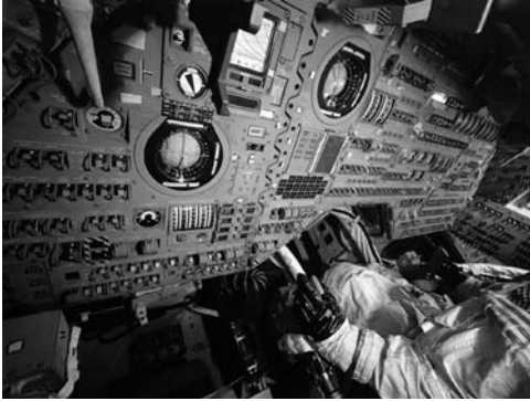
The large main display console in the CM that stretched from one side of the cabin to the other.
