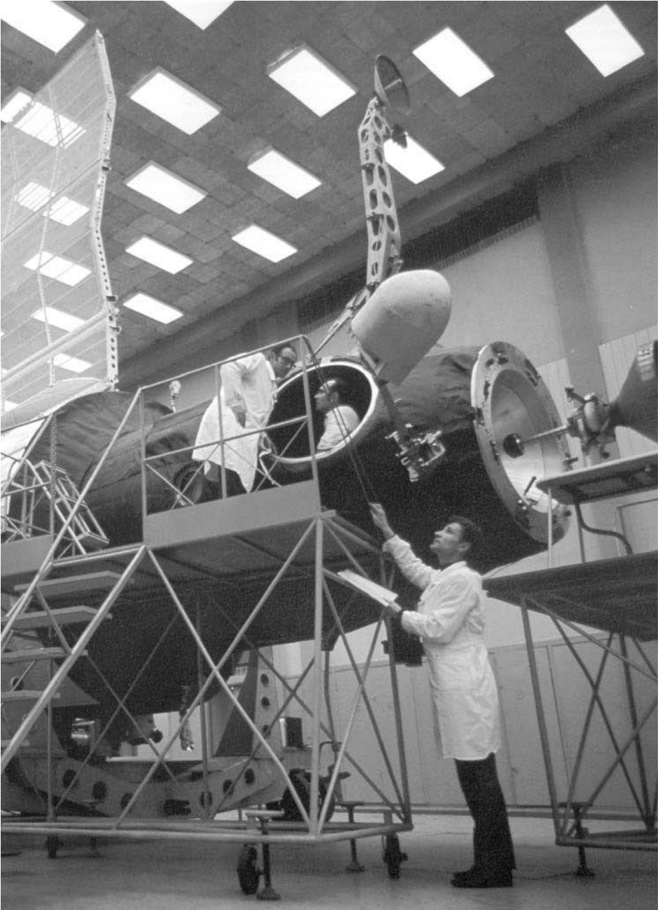
Inspecting the DOS-3 simulator. Note the Soyuz docking probe on the right.
