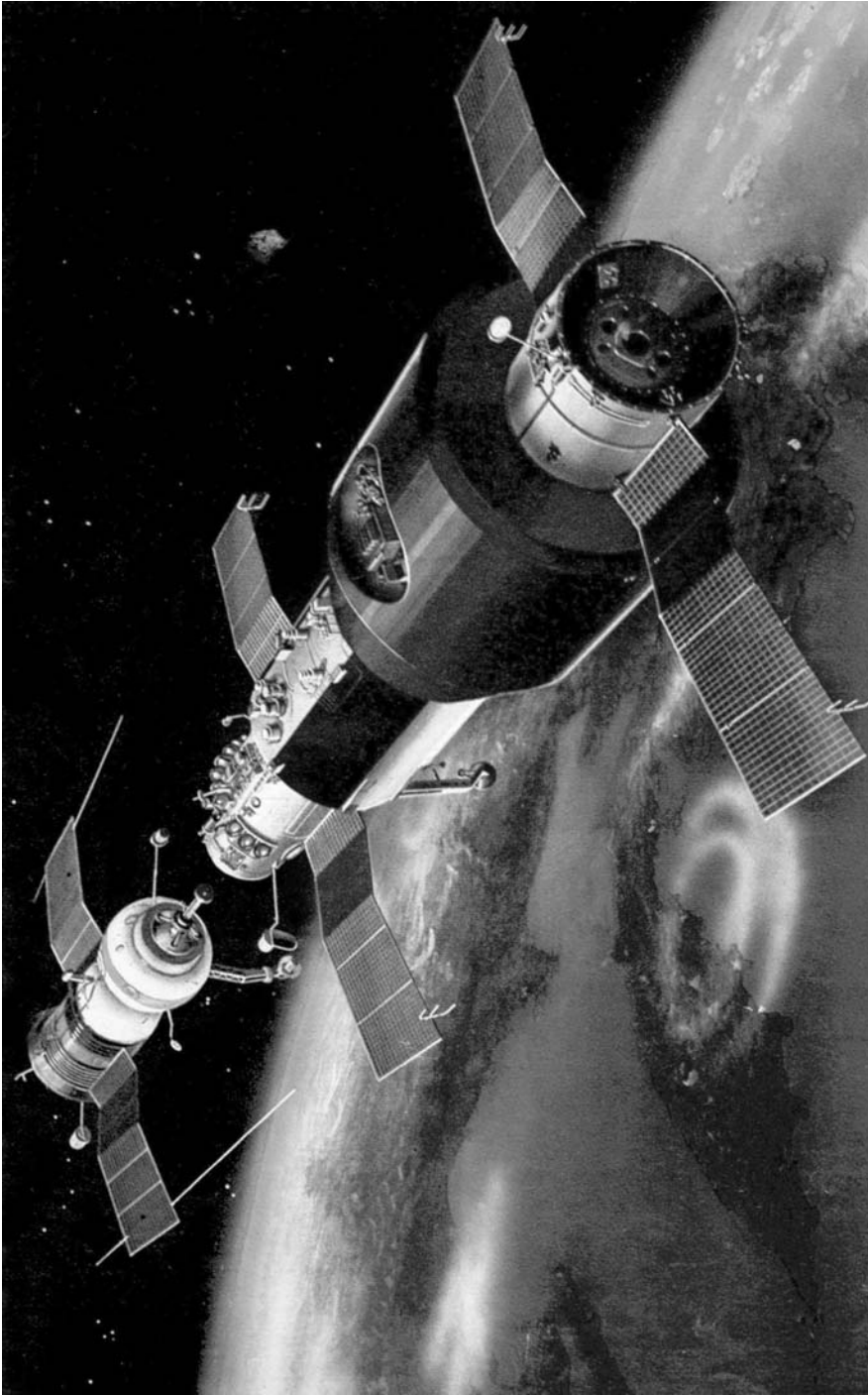
An accurate painting of Soyuz 11 about to dock with the Salyut space station above the Kamchatka peninsula. Although the scientific instrument aperture on the main compartment is shown facing away from the Earth, in fact the protective cover had failed to release, rendering the instruments unusable. (Painting by Andrey Sokolov and cosmonaut Aleksey Leonov)
