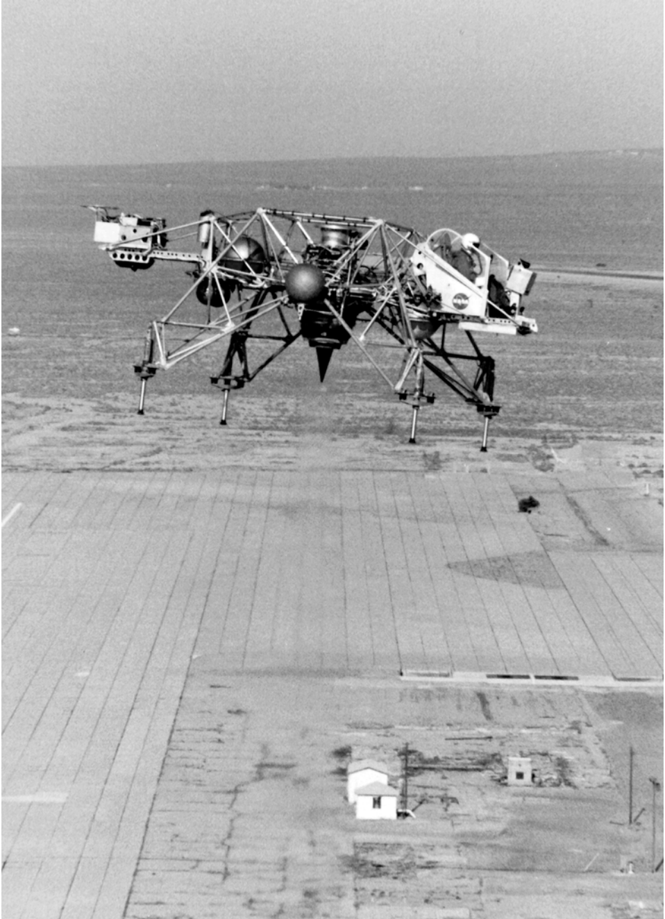
The Lunar Landing Research Vehicle in 1965 at its maximum altitude during a test flight at Edwards Air Force Base.
