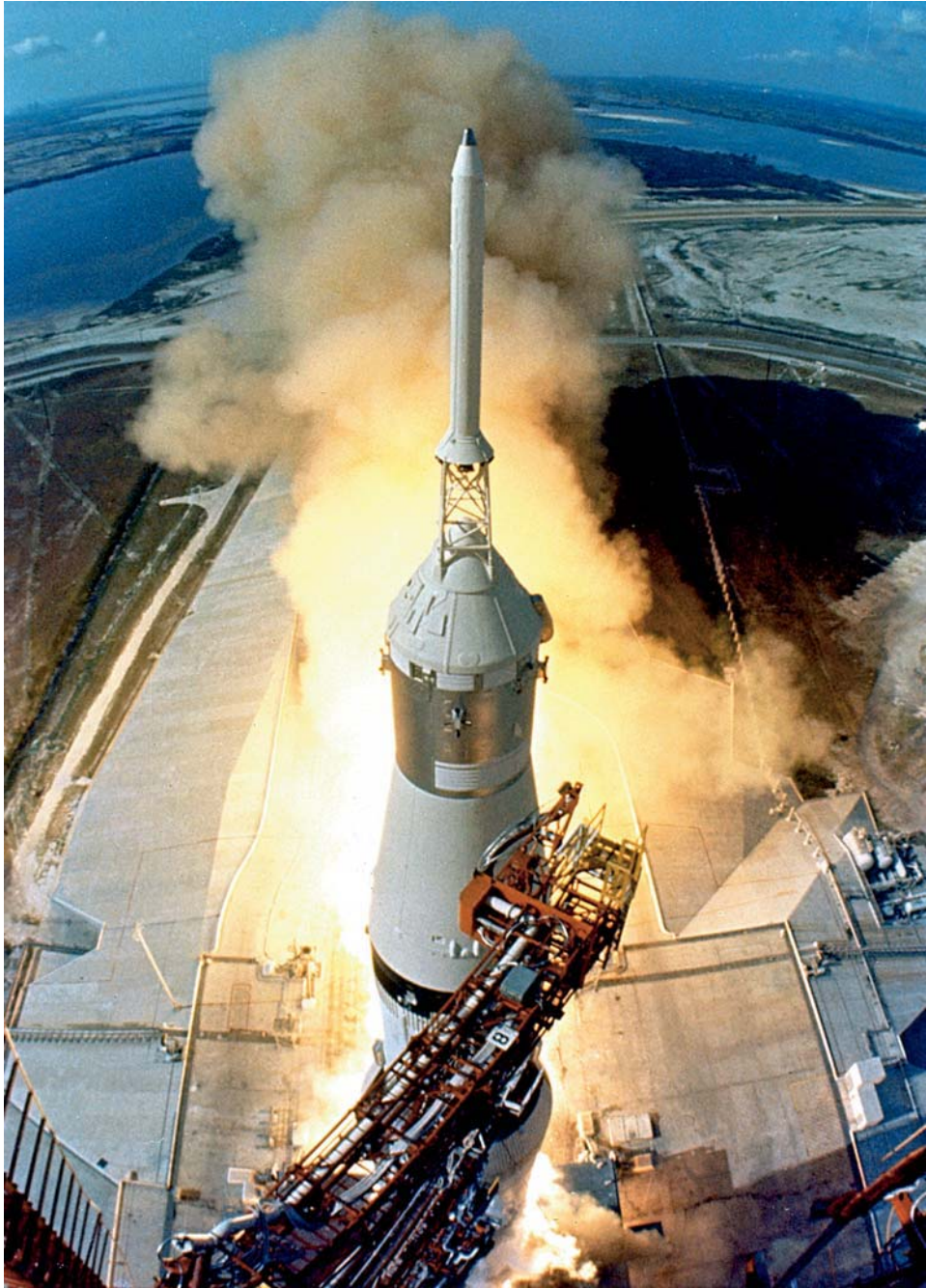
As Apollo 11 lifts off, the lower arms of the tower swing away.
