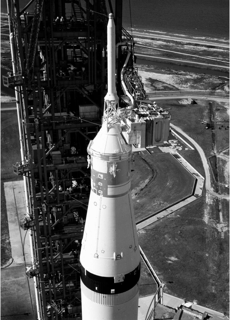
The White Room on Swing Arm 9 provided access to the spacecraft.
