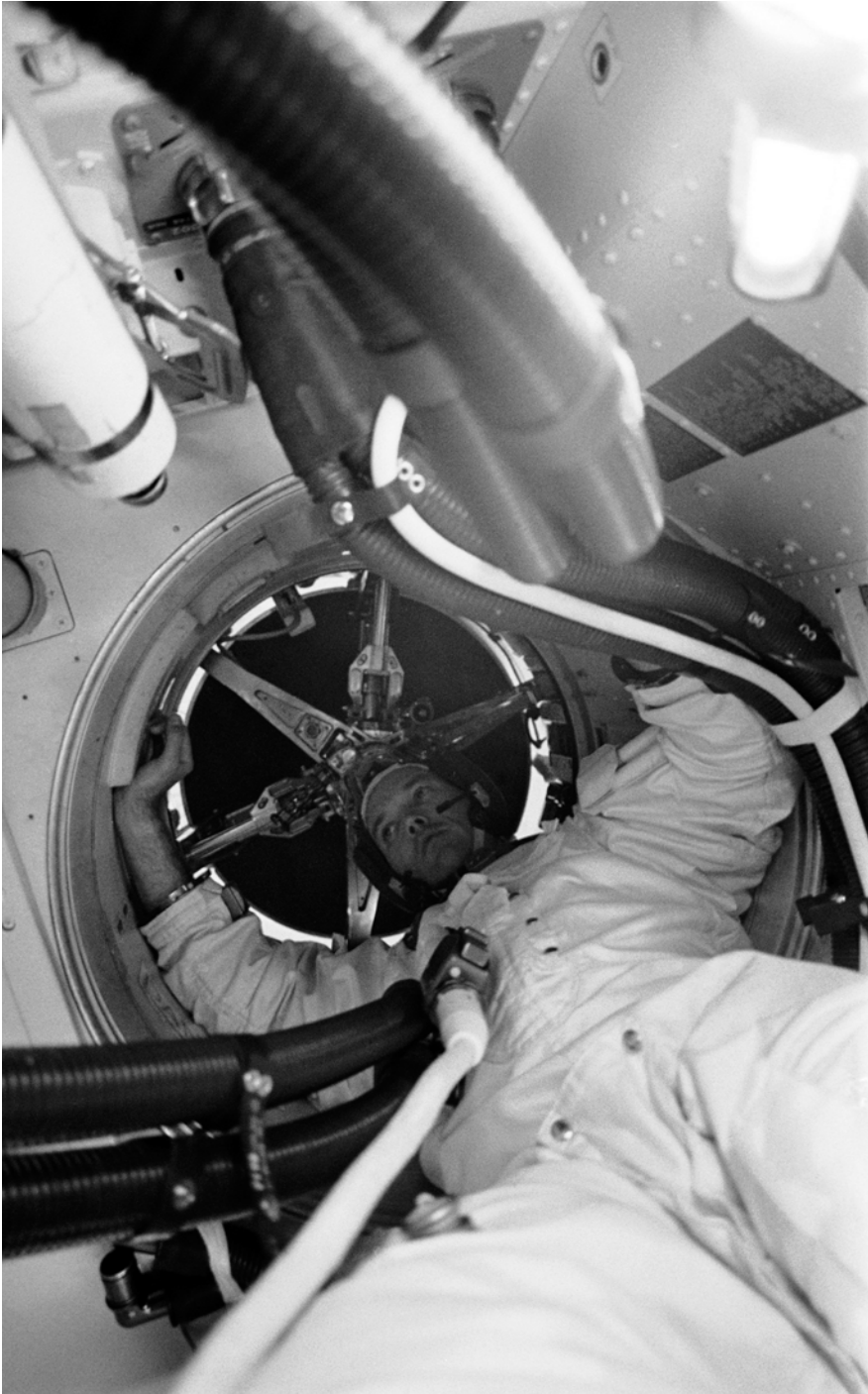
Having removed the apex hatch, Mike Collins prepares to remove the probe assembly.
