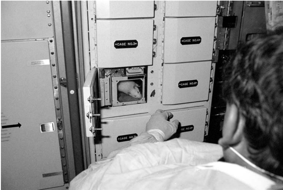
Taken during STS 51-B, this photograph shows how the animal enclosure modules (AEMs) were positioned inside lockers on the shuttle's mid-deck. Mission specialist Norm Thagard is checking on the rodents in one AEM. (Photo: NASA)
