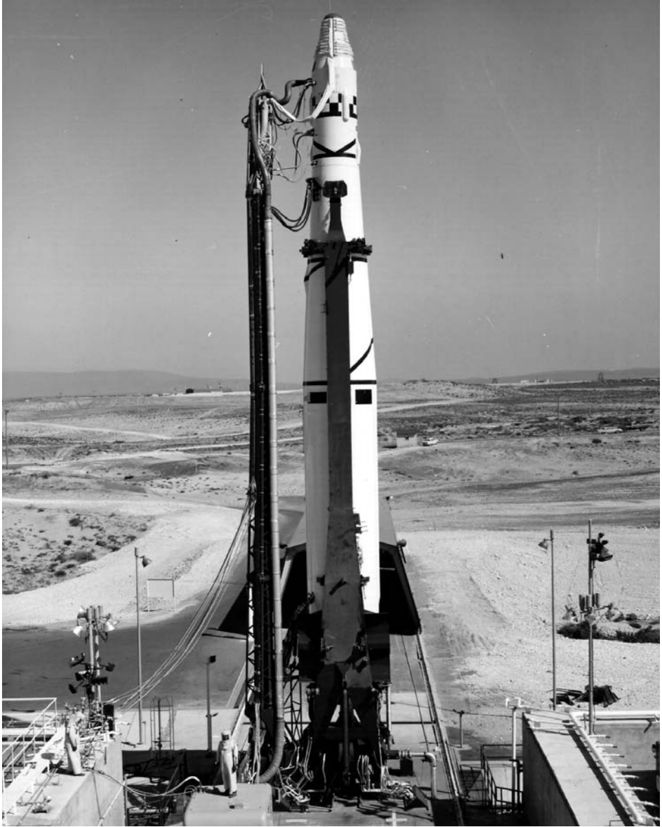
The Thor-Agena combination used in Discoverer launches. (Photo: USAF)
