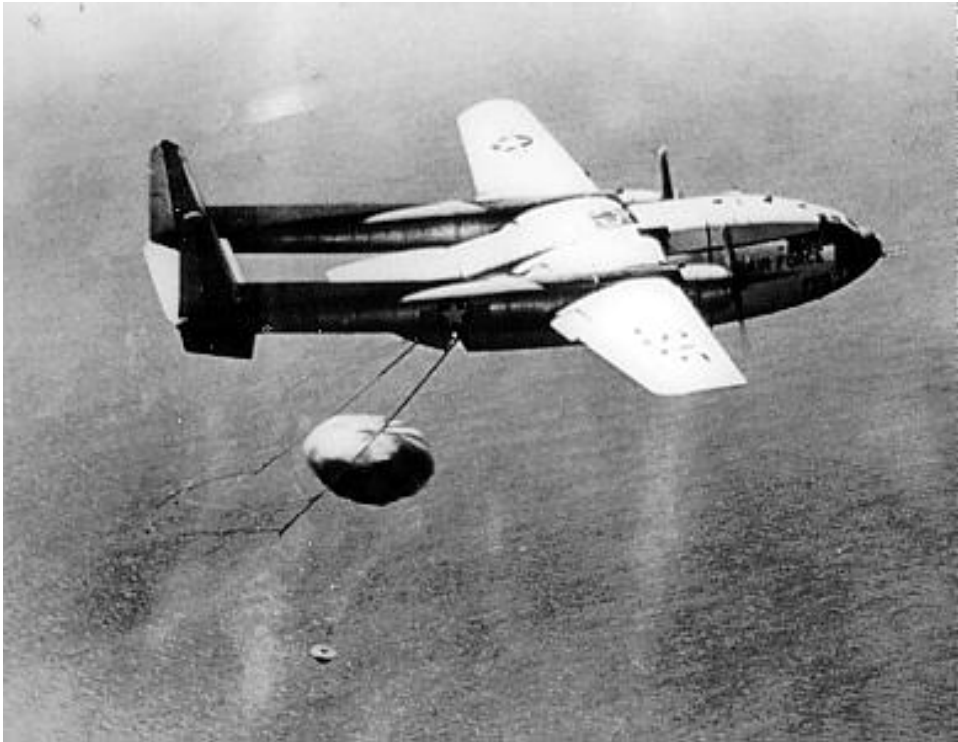
Discoverer XIV's bucket is snagged by a C-119 aircraft under the command of Captain Harold E. Mitchell. (Photo: USAF)
