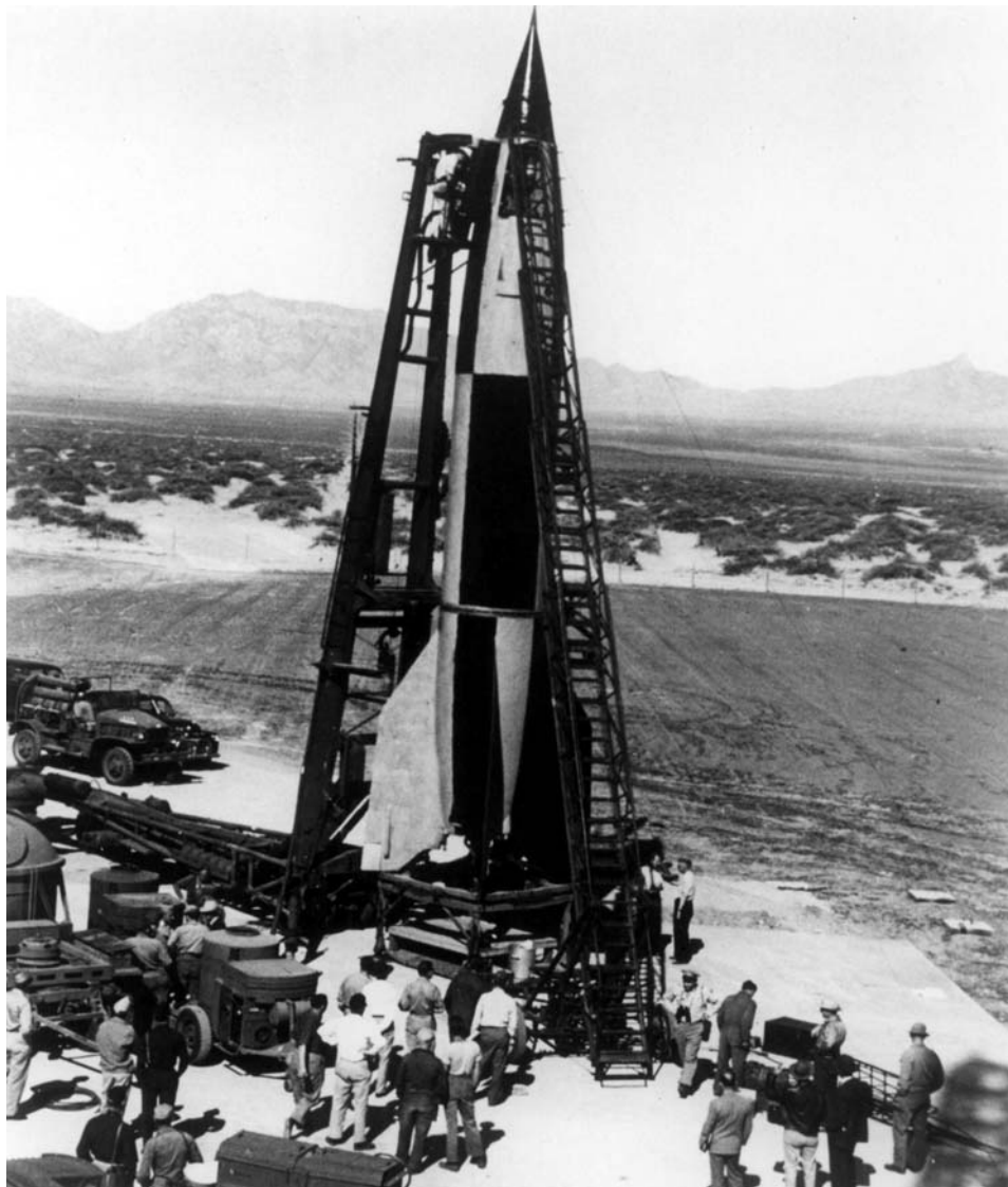
Loading alcohol fuel aboard a V-2 before firing from the U.S. Army Ordnance Proving Ground at White Sands, New Mexico. Note the use of a ladder to top up the fuel. (Photo: U.S. Army)
