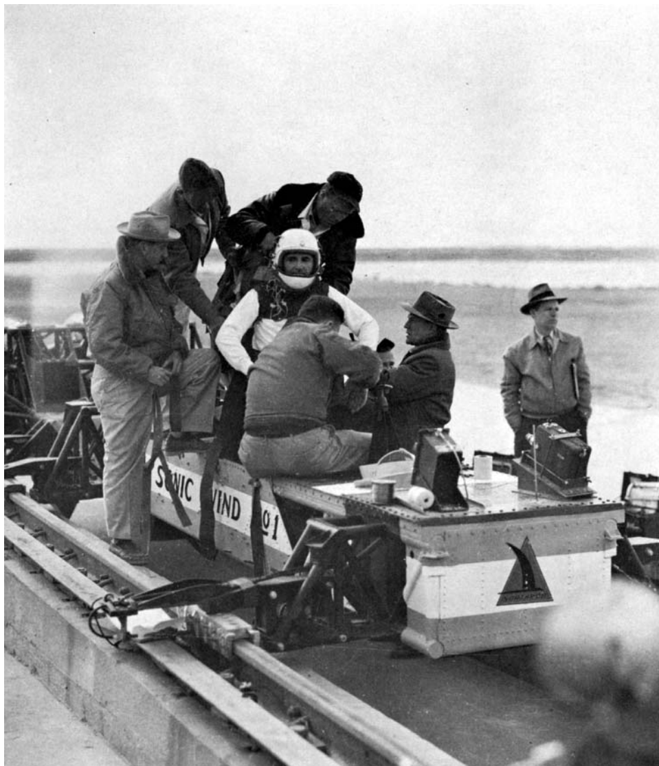
Lt. Colonel John Paul Stapp aboard Sonic Wind No. 1 prepares for a rocket-powered sled ride to test the effects of acceleration and deceleration research. (Photo: USAF)
