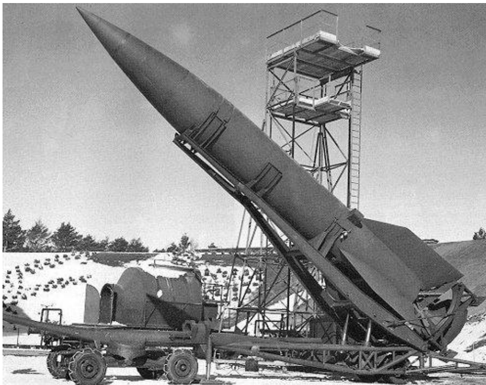
A wooden mock-up of a V-2 rocket is shown loaded on a meillerwagen hydraulic transporter in February 1942. (Photo: U.S. Army)
