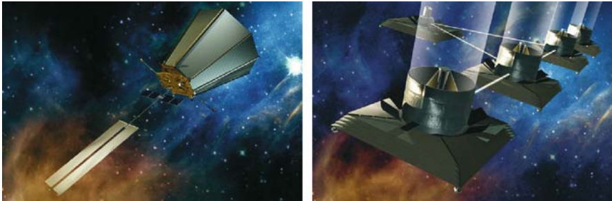
Fig. 4.9. The Terrestrial Planet Finder TPF comprises two complementary observatories: a visible-light coronagraph TPF-C ( left ), to be launched around 2014, and a formation-flying infrared interferometer TPF-I, to be launched before 2020 (courtesy of NASA)
