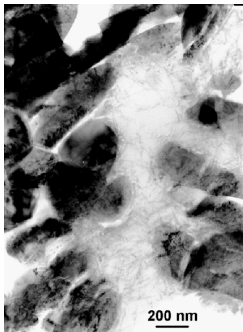
Fig. 3.9. Transmission electron microscope micrograph of an ultra-microtomed section of a Cap-Prudhomme Antarctic micrometeorite. The fibrous material filling the voids between crystals is very likely made of “nanotubes” of ferrihydrite. The associated electron diffraction pattern clearly shows that they are made of ferrihydrite (Courtesy G. Matrajt).
