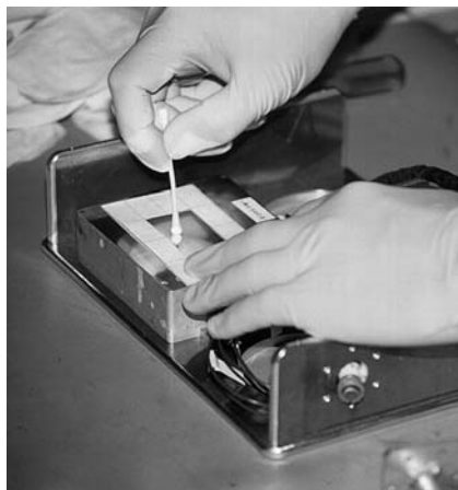
Fig. 13.1 Swabbing of an area ( 5 \times 5 \text{ cm}^2 ) of a spacecraft subunit of the Mars '96 mission (photo credit: CNES).
