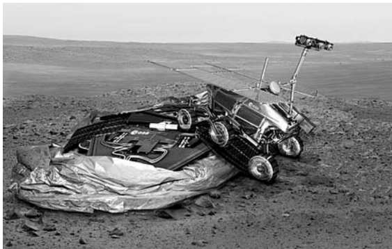
Fig. 12.7 Artist's representation of the ExoMars rover's egress from the descent module (image credit: ESA).
