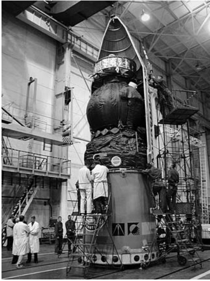
Fig. 11.9 Final assembly of Foton with the Soyuz nosecone. BIOPAN is visible on the top of the descent module (photo credit: ESA).
