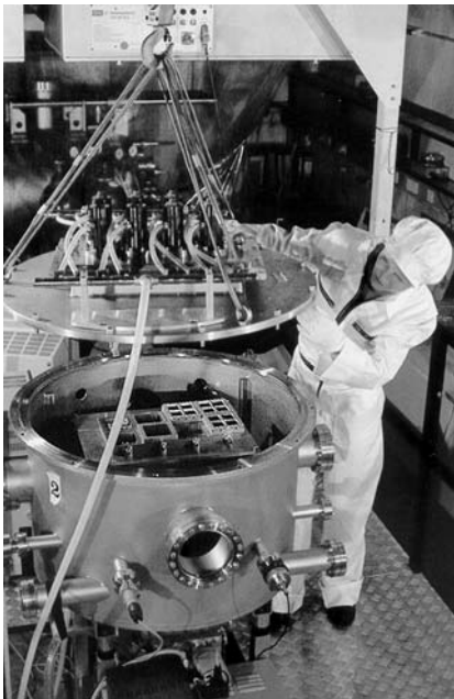
Fig. 11.19 Space Simulation Facility (PSI) at the Institute of Aerospace Medicine, DLR, for the pre-flight testing of the experiments on EURECA and EXPOSE (photo credit: DLR).
