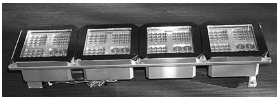
Fig. 11.14 One of the three trays of EXPOSE; photo of the Engineering Model (courtesy of ESA).
