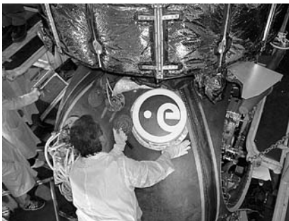
Fig. 11.7 Installation of BIOPAN onto the descent module of the satellite Foton , during the pre-launch operations (photo credit: ESA).
