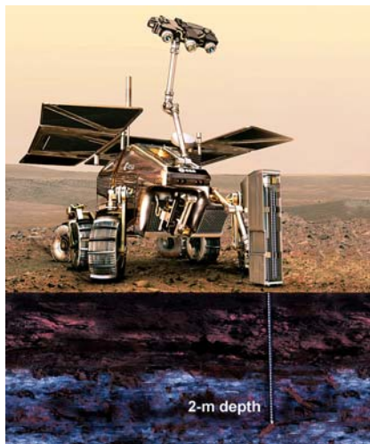
Fig. 12.9 Artist's view of the ExoMars rover with the drill obtaining a sample from the Martian subsurface (image credit: ESA).
