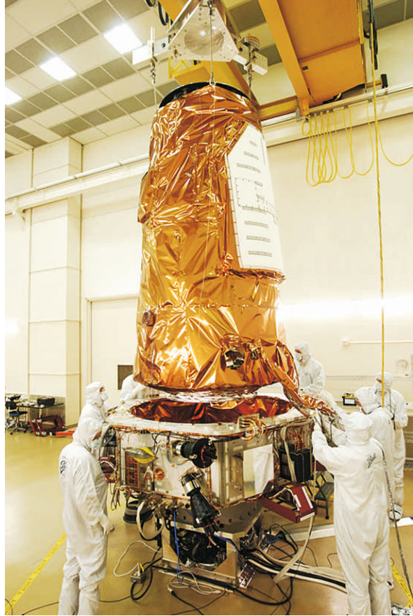
Fig. 6.4 The Kepler telescope which is mainly used as a photometer to observe simultaneously the brightness of 100 000 stars using 42 CCD cameras. Credit: NASA, Kepler mission
