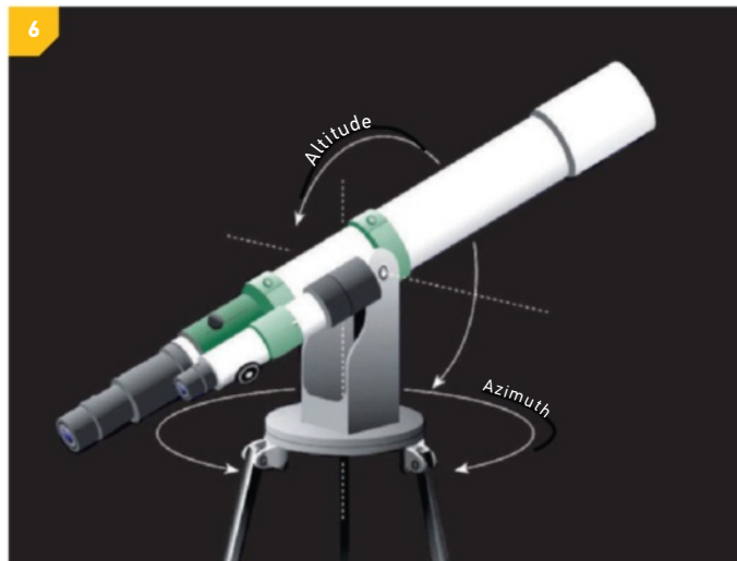
6 A basic alt-az mount provides side-to-side and up-and-down motion.
