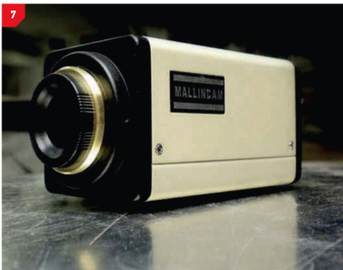
[7] Integrating video camera used for low-light astrovideo.
