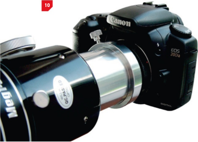
[10] DSLR camera prime-focus coupled to a telescope.
